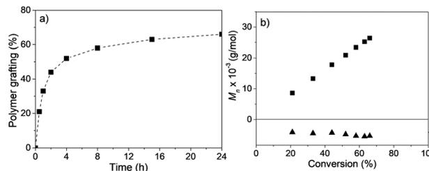
Fig. 4 (a) Evolution of %polymer grafting into the mesopores of MSN-Br vs. time and (b) plot of  $M_n$  and  $D$  of the cleaved polymer vs. %polymer grafting for SC-ATRP of AN + 15% VBC in xylene at 90 °C.
