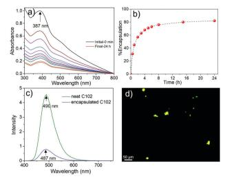
Fig. 6 (a) Time-dependent (initial - 0 min, final - 24 h) UV-Vis spectra of C102 after incubating with NMCN; (b) evaluation of %encapsulation of C102 with time; (c) fluorescence emission spectra of aqueous solution of C102 and aqueous suspension of C102 encapsulated-NMCN (Excitation wavelength: 390 nm); (d) fluorescent microscopy images of C102 encapsulated-NMCN.
