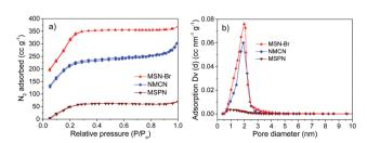
Fig. 2 (a) N<sub>2</sub> adsorption-desorption isotherm and (b) pore size distribution of porous MSN-Br, MSPN and NMCN nanomaterials.
