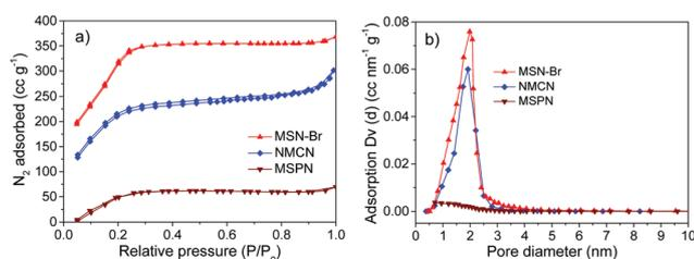
Fig. 2 (a) N<sub>2</sub> adsorption-desorption isotherm and (b) pore size distribution of porous MSN-Br, MSPN and NMCN nanomaterials.
