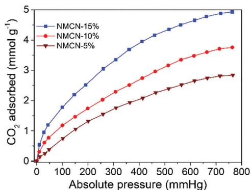
Fig. 5 CO<sub>2</sub> adsorption isotherms for NMCN samples at 25 °C.
