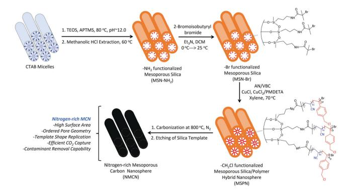
Scheme 1 Synthesis of nitrogen-rich mesoporous carbon nanoparticles.
