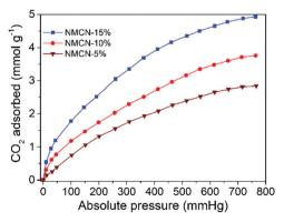
Fig. 5 CO<sub>2</sub> adsorption isotherms for NMCN samples at 25 °C.
