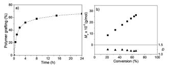
Fig. 4 (a) Evolution of %polymer grafting into the mesopores of MSN-Br  $\emph{vs.}$  time and (b) plot of  $\emph{M}_{n}$  and  $\emph{D}$  of the cleaved polymer  $\emph{vs.}$  %polymer grafting for SC-ATRP of AN + 15% VBC in xylene at 90 °C.
