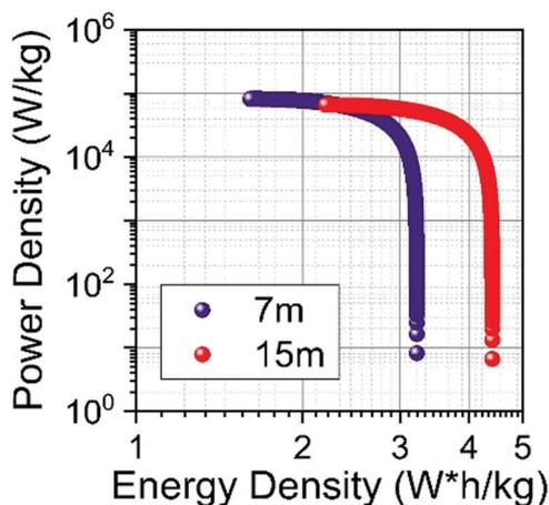
Fig. 12 Ragone plot for symmetrical supercapacitors filled with SiWE (7 mol kg<sup>-1</sup>) and WiSE NaClO<sub>4</sub> (15 mol kg<sup>-1</sup>) solutions. Electrodes: MWCNTs.
