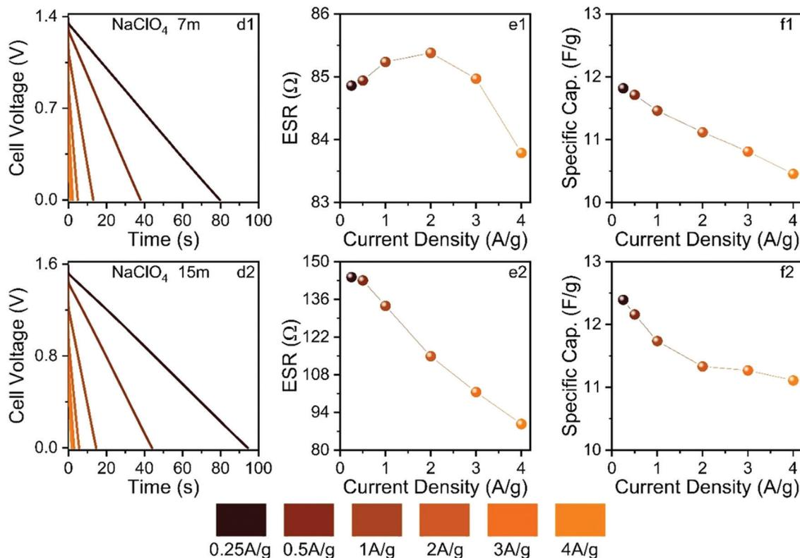
Fig. 11 Findings from the galvanostatic charge–discharge experiments obtained for (1) 7 mol kg<sup>-1</sup> and (2) 15 mol kg<sup>-1</sup> NaClO<sub>4</sub> aqueous solutions. Plots: (d1 & d2) discharge curves, (e1 & e2) equivalent series resistance, and (f1 & f2) specific capacitance as a function of the applied current density in the range of 0.25 A g<sup>-1</sup> to 4 A g<sup>-1</sup>. Electrode: MWCNTs.
