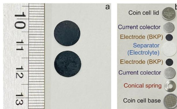
**Fig. 2** (a) Self-supporting MWCNT electrodes. (b) Components of a symmetric supercapacitor assembled using a model CR 2032 coin cell filled with the SiWE (7 mol kg<sup>-1</sup>) or WiSE (15 mol kg<sup>-1</sup>) NaClO<sub>4</sub> solutions.
