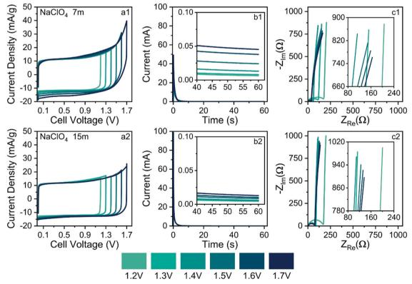
Fig. 10 Electrochemical findings obtained using the CV (a), SSC (b), and EIS (c) techniques. Conditions: (a-c)(1) 7.0 mol kg<sup>-1</sup> NaClO<sub>4</sub>, and (a-c)(2) 15.0 mol kg $^{-1}$  NaClO<sub>4</sub>.  $\nu$  = 1 mV s $^{-1}$ . Electrode: MWCNTs.
