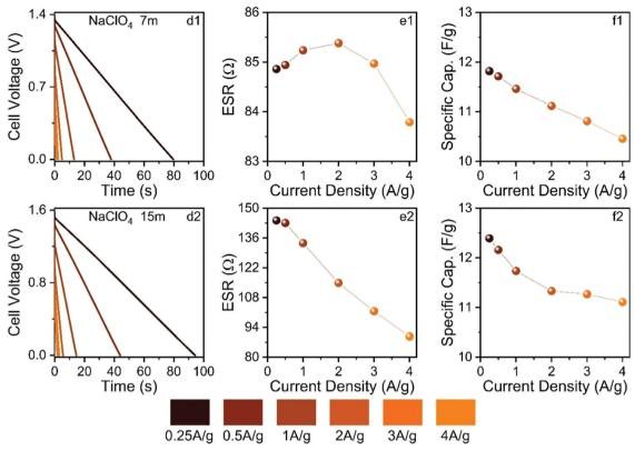
Fig. 11 Findings from the galvanostatic charge-discharge experiments obtained for (1) 7 mol kg $^{-1}$  and (2) 15 mol kg $^{-1}$  NaClO<sub>4</sub> aqueous solutions. Plots: (d1 & d2) discharge curves, (e1 & e2) equivalent series resistance, and (f1 & f2) specific capacitance as a function of the applied current density in the range of 0.25 A  $g^{-1}$  to 4 A  $g^{-1}$ . Electrode: MWCNTs.
