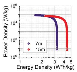
Fig. 12 Ragone plot for symmetrical supercapacitors filled with SiWE (7  $mol kg^{-1}$ ) and WiSE NaClO<sub>4</sub> (15  $mol kg^{-1}$ ) solutions. Electrodes: MWCNTs.
