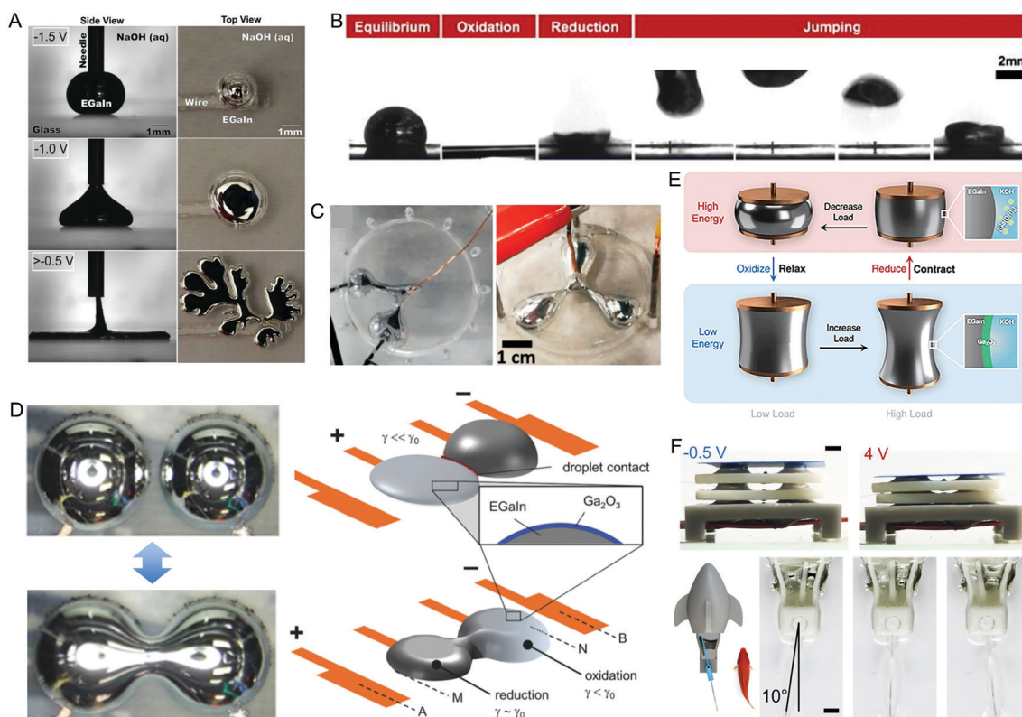
Fig. 2 Actuators enabled by oxidation and reduction of LM. (A) Oxidation of LM immersed in NaOH solution causes its interfacial tension to reduce significantly, resulting in flattening and spreading of the LM. Reproduced with permission. 38 Copyright 2014, National Academy of Sciences. (B) A LM droplet jumps over 5 mm high due to oxidation and reduction. Reproduced with permission. 52 Copyright 2021, American Institute of Physics. (C) LM shape control using electrochemistry. Reproduced with permission. 54 Copyright 2019, MDPI. (D) Merging and separation of LM used as an electrical switch. Reproduced with permission. 55 Copyright 2017, Wiley-VCH. (E) A LM artificial muscle with copper pads on either side to pin the LM. Contraction and relaxation of the LM artificial muscle can be achieved upon oxidation or reduction. Reproduced with permission. 57 Copyright 2021, Royal Society of Chemistry. (F) Actuation of a 3-layer stack LM artificial muscle and using a LM artificial muscle to swing the caudal fin of an untethered bionic robotic fish. Scale bars are 2 mm. Reproduced with permission. 56 Copyright 2021, Wiley-VCH.
