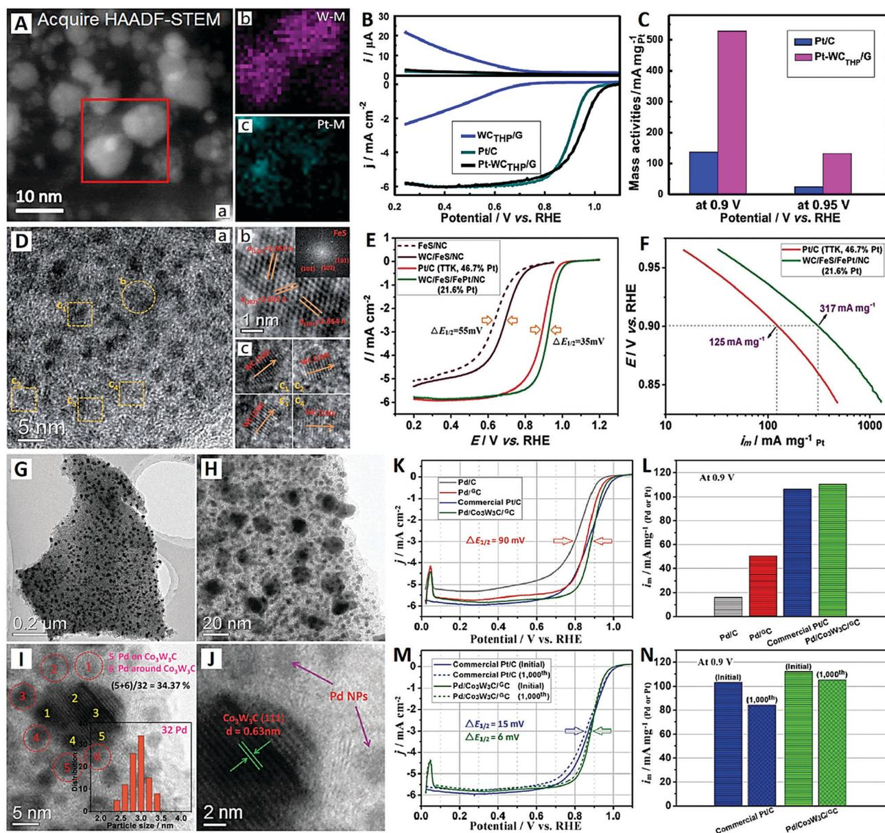
Fig. 5 The Pt-WC<sub>THP</sub>/G catalyst (reprinted with permission from ref. 93): (A) HAADF-STEM images and (B and C) electrochemical performances. The WC/FeS/FePt/NC catalyst (reprinted with permission from ref. 94): (D) TEM images and (E and F) electrochemical performances. The Pd/Co<sub>3</sub>W<sub>3</sub>C/GC catalyst (reprinted with permission from ref. 95): (G–J) TEM images and (K–N) electrochemical performances.
