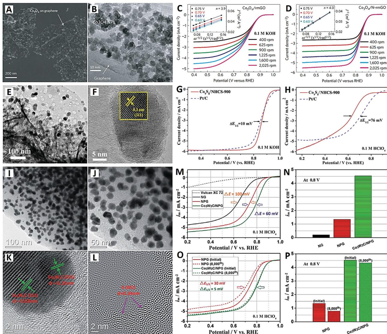
Fig. 4 The  $\text{Co}_3\text{O}_4/\text{N-rmGO}$  catalyst (reprinted with permission from ref. 84): (A and B) SEM and TEM images, and (C and D) electrochemical performances. The  $\text{Co}_9\text{S}_8/\text{NHCS-900}$  catalyst (reprinted with permission from ref. 85): (E and F) TEM images and (G and H) electrochemical performances. The  $\text{Co}_3\text{W}_3\text{C}/\text{NPG}$  catalyst (reprinted with permission from ref. 88): (I–L) TEM images and (M–P) electrochemical performances.
