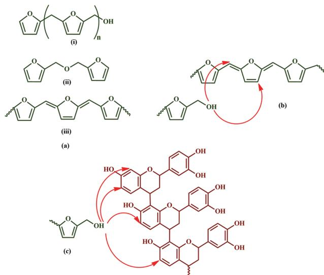
**Fig. 19** (a) Self-condensation of furfuryl alcohol: (i) chain condensation reaction, (ii) reaction between hydroxyl groups and (iii) rearrangement of furanic cycle; (b) crosslinking sites for furfuryl alcohol; (c) possible reaction sites between flavonoid units and polyfurfuryl alcohol's hydroxyl group.
