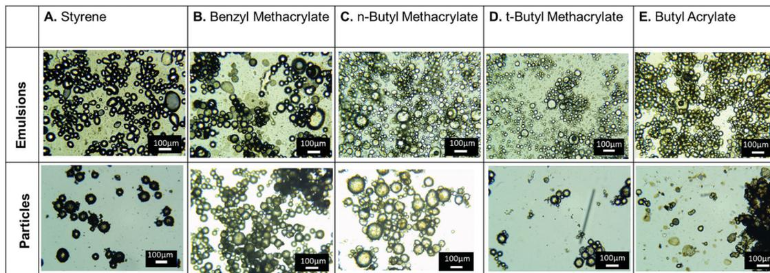
Fig. 3 Optical microscopy images of emulsions (top) stabilized by salt-flocculated CONs and their respective CON-armed particles (bottom) prepared using: (A) styrene, (B) benzyl methacrylate, (C) *n*-butyl methacrylate, (D) *t*-butyl methacrylate, and (E) *n*-butyl acrylate.  $1.2 \text{ mg mL}^{-1}$  of flocculated CONs and  $0.0025 \text{ M NaCl}$  were used.
