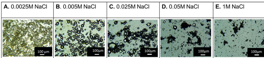
Fig. 2 Styrene-in-water emulsions stabilized by CONs flocculated with (A) 0.0025 M NaCl, (B) 0.005 M NaCl, (C) 0.025 M NaCl, (D) 0.05 M NaCl, and (E) 0.1 M NaCl. An aqueous dispersion of  $1.2 \text{ mg mL}^{-1}$  of CONs was used and a 1 : 5 oil : water ratio.
