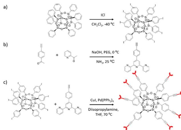
**Scheme 1** (a) Synthesis of I-POSS, (b) synthesis of 4'-(4-ethynylphenyl)-[2,2':6,2'']terpyridine, and (c) synthesis of novel POSS (Ter-POSS) *via* a Sonogashira reaction.
