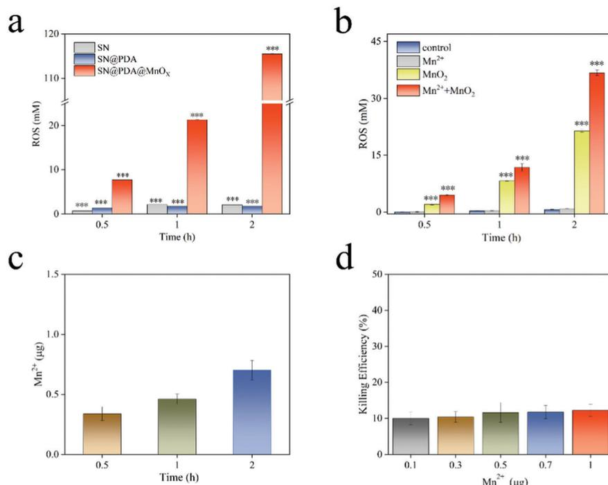
**Fig. 5** (a) ROS generation of SN, SN@PDA, SN@PDA@MnO<sub>x</sub> immersed in PBS for different time. (b) The effect of Mn<sup>2+</sup> and MnO<sub>2</sub> on the generation of ROS from SN@PDA. (c) The release of Mn<sup>2+</sup> from SN@PDA@MnO<sub>x</sub>. (d) Bacterial killing efficiency of Mn<sup>2+</sup>. The data were expressed as mean ± SD, *n* = 3, \*\*\**p* < 0.001, 0 h (a) and SN@PDA (b) were used as a control group for significant difference analysis.
