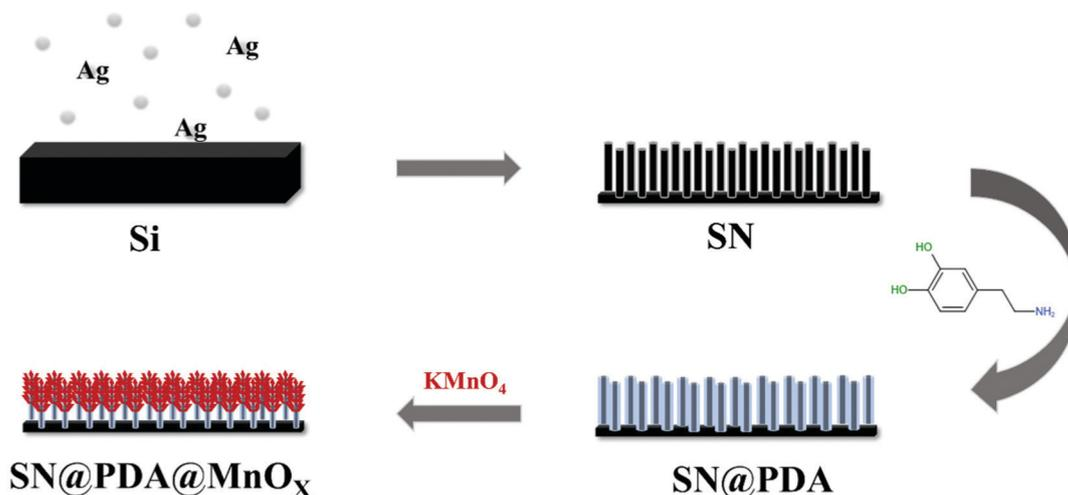
Fig. 1 Preparation of SN@PDA@MnO<sub>x</sub>.
