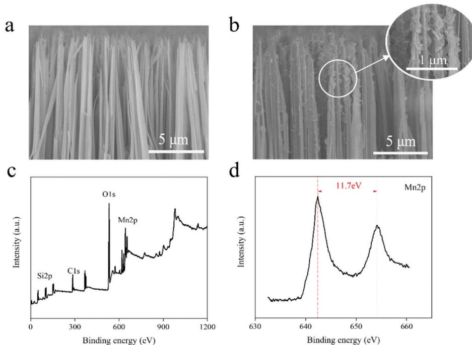
Fig. 2 (a) SEM image of SN (cross section). (b) SEM image of SN@PDA@MnO<sub>x</sub> (cross section). (c) XPS full spectrum of SN@PDA@MnO<sub>x</sub>. (d) XPS narrow scan of SN@PDA@MnO<sub>x</sub> for Mn.
