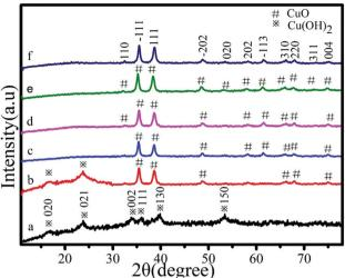
Fig. 4 XRD patterns of the leaf-like copper oxide mesocrystals obtained by collagen-templated biomineralization ([collagen] = 0.5 wt%, [Cu(II)] = 0.02 mol L<sup>-1</sup>) after different incubation times: (a) 0.5 hours; (b) 1.5 hours; (c) 3 hours: (d) 6 hours: (e) 9 hours: and (f) 12 hours
