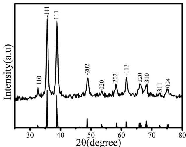
Fig. 1 XRD pattern of the as-prepared copper oxide particles obtained via collagen-templated biomineralization ([collagen] = 0.5 wt%, [Cu(II)] = 0.02 mol  $\text{L}^{-1}$ ). The standard XRD pattern (copper oxide, JCPDS no. 05-0661) is shown beneath the plot.
