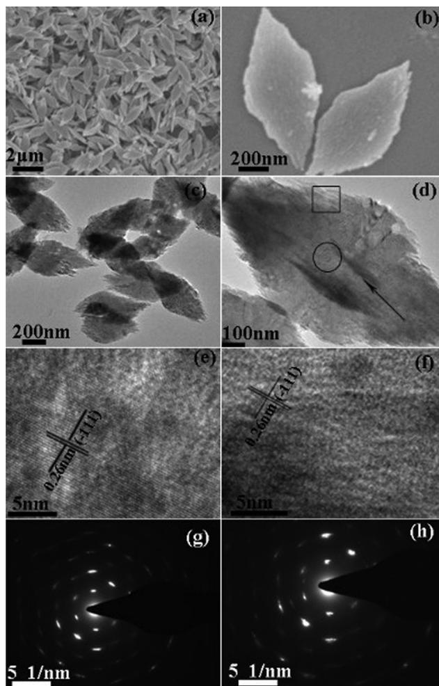
Fig. 2 (a and b) FESEM images of the leaf-like copper oxide mesocrystals obtained after 12 hours via collagen-templated biomineralization ([collagen] = 0.5 wt%, [Cu(II)] = 0.02 mol L<sup>-1</sup>); (c and d) TEM images of the same copper oxide particles; (e) HRTEM image of the circle part of (d); and (f) HRTEM image of the square part of (d). (g) SAED pattern of the circle part of (d); and (h) SAED pattern of the square part of (d).
