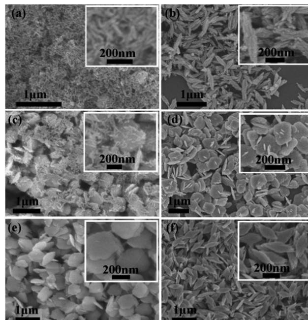
Fig. 3 FESEM images of the leaf-like copper oxide mesocrystals obtained by collagen-templated biomineralization ([collagen] = 0.5 wt%, [Cu(II)] = 0.02 mol L<sup>-1</sup>) after different incubation times: (a) 0.5 hour; (b) 1.5 hours; (c) 3 hours; (d) 6 hours; (e) 9 hours; and (f) 12 hours.
