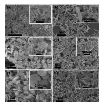
**Fig. 3** FESEM images of the leaf-like copper oxide mesocrystals obtained by collagen-templated biomineralization ([collagen] = 0.5 wt%, [Cu(III)] = 0.02 mol L $^{-1}$ ) after different incubation times: (a) 0.5 hour; (b) 1.5 hours; (c) 3 hours; (d) 6 hours; (e) 9 hours; and (f) 12 hours.
