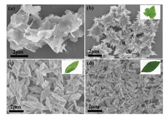
Fig. 5 FESEM images of copper oxide mesocrystals obtained after 12 hours via collagen-templated biomineralization with a constant Cu(II) concentration (0.02 mol  $L^{-1}$ ) and varying concentrations of collagen: (a) 0, (b) 0.05, (c) 0.2, and (d) 0.5 wt%.
