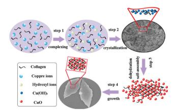
Scheme 1 Illustration of the critical role of collagen in the mediation of hierarchical nanostructures of copper oxide mesocrystals.
