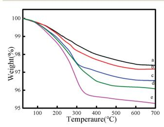
Fig. 6 TGA curves of CuO samples synthesized under various concentrations of collagen: (a) 0, (b) 0.05, (c) 0.1, (d) 0.2, and (e) 0.5 wt%.
