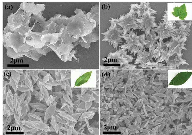
Fig. 5 FESEM images of copper oxide mesocrystals obtained after 12 hours *via* collagen-templated biomineralization with a constant Cu(II) concentration (0.02 mol L<sup>-1</sup>) and varying concentrations of collagen: (a) 0, (b) 0.05, (c) 0.2, and (d) 0.5 wt%.
