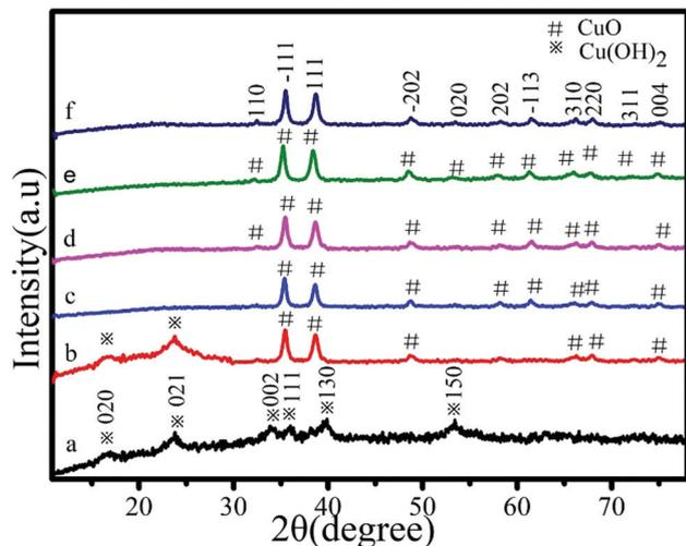
Fig. 4 XRD patterns of the leaf-like copper oxide mesocrystals obtained by collagen-templated biomineralization ([collagen] = 0.5 wt%, [Cu(II)] = 0.02 mol L<sup>-1</sup>) after different incubation times: (a) 0.5 hours; (b) 1.5 hours; (c) 3 hours; (d) 6 hours; (e) 9 hours; and (f) 12 hours.
