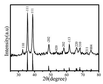
Fig. 1 XRD pattern of the as-prepared copper oxide particles obtained via collagen-templated biomineralization ([collagen] = 0.5 wt%, [Cu(II)] =  $0.02 \text{ mol L}^{-1}$ ). The standard XRD pattern (copper oxide, JCPDS no. 05-0661) is shown beneath the plot
