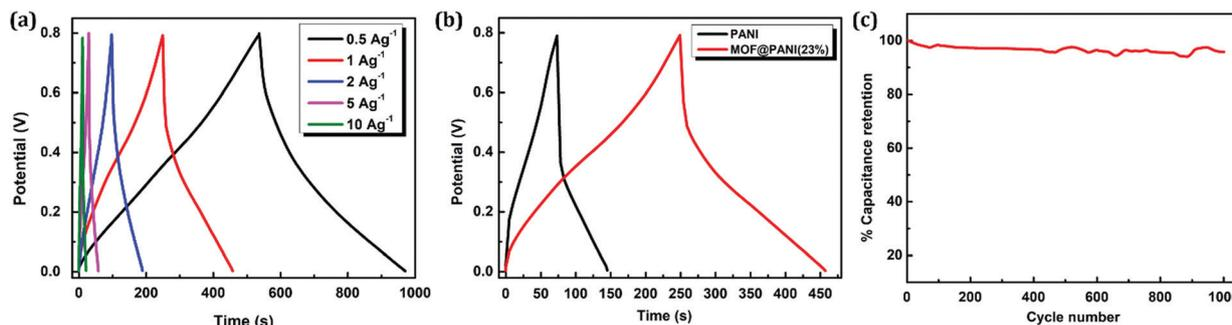
Fig. 7 Two-electrode setup characterization of the MOF@PANI (23 wt%) showing (a) the GCD profile at different charging current density for the MOF@PANI\_23 wt%, (b) GCD response comparison with PANI at a current density of 1 A g<sup>-1</sup>, and (c) capacitance retention over 1000 cycles.
