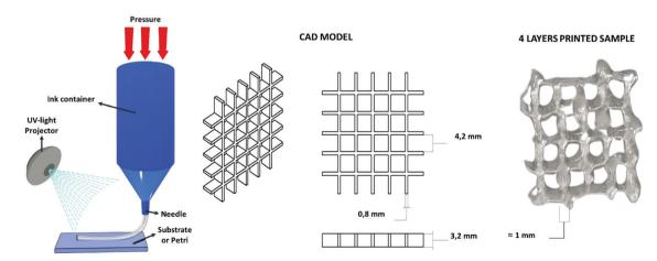
Fig. 6 Extrusion-based 3D printing scheme, the used CAD model and the four-layer grid immediately after printing
