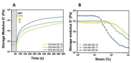
Fig. 4 Photo-rheology (A) and amplitude sweep (B) of CHI-MA at different %DS.
