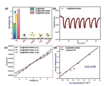
Fig. 9 (a) Selectivity towards exposure to interfering gases and (b) repeatability of 1D aligned co-axial CFs@NiNPs-PtNPs towards H2 at room temperature, (c) current-voltage characteristics of co-axial CFs@NiNPs-PtNPs under N2, H2 and air atmospheres and (d) sensor response as a function of (hydrogen concentration)<sup>1/2</sup> at RT.
