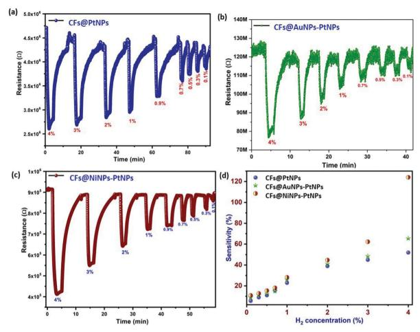
Fig. 8 Dynamic H<sub>2</sub> gas sensing properties of 1D aligned co-axial (a) CFs@PtNPs, (b) CFs@AuNPs-PtNPsAuNPs-PtNPs and (c) CFs@NiNPs-PtNPs. (d) Comparative sensitivity as a function of H2 concentration of 1D aligned co-axial CFs@PtNPs, CFs@AuNPs-PtNPs and CFs@NiNPs-PtNPs
