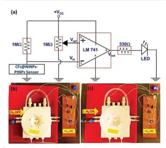
Fig. 11 Real-time demonstration of the proposed 1D aligned co-axial CF@NiNP-PtNP sensor: (a) equivalent electronic circuit diagram. Photograph of the prototype sensor device during (b) H2 OFF state and (c) H2 ON
