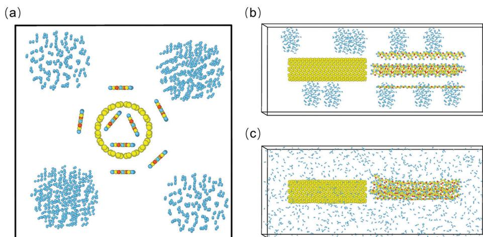
**Fig. 1** The initial model consisting of hydrogen, (10, 10) SWCNTs, and PT chains. (a) A top view and (b) side view. (c) A snapshot of the simulation box (side view) after a simulation time of 0.5 ns. Blue, yellow, and red represent H, C, and S atoms, respectively.
