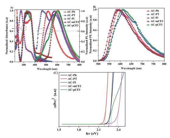
Fig. 2 (A) UV absorption and PL spectra of dyes in CHCl<sub>3</sub> solution, (B) PL spectra of dyes in solid and (C) optical bandgap of the dyes calculated from the solid-state diffuse reflectance spectra.
