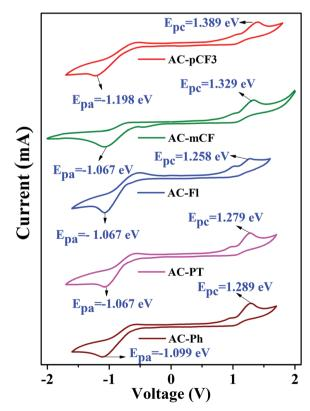
Fig. 8 Cyclic voltammograms of the AC-derivatives.
