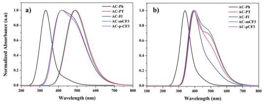
Fig. 7 UV-Visible spectra of AC-derivatives in gas (a) and DCM (b) phase.
