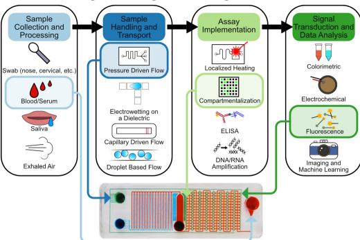
Fig. 1 Overview and selection of the various components that contribute to forming an integrated microfluidic chip for diagnostics. Example chip: the SIMPLE chip.<sup>19</sup> Reproduced/adapted from ref. 19 with permission from Science.
