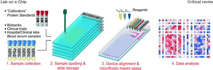
Fig. 4 An illustration of the workflow for the parallel immunoassay. Clinical samples are spotted with a microarray robot on the same array as protein standards. The microfluidic device is aligned to the array and proper tubing is connected. The chip is then run the next day and the subsequent data is be analyzed. Reproduced/adapted from ref. 119 with permission from the Royal Society of Chemistry.
