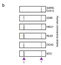
Fig. 2 Image of lateral flow assay in a mask for aerosol sample collection. (a) Photos of a SARA-CoV-2 sensor in a mask. (b) Representative images of the LFA outputs for various human coronovirus strains. Images adapted with permission from ref. 41. Copyright © (2021) Nature Publishing Group.
