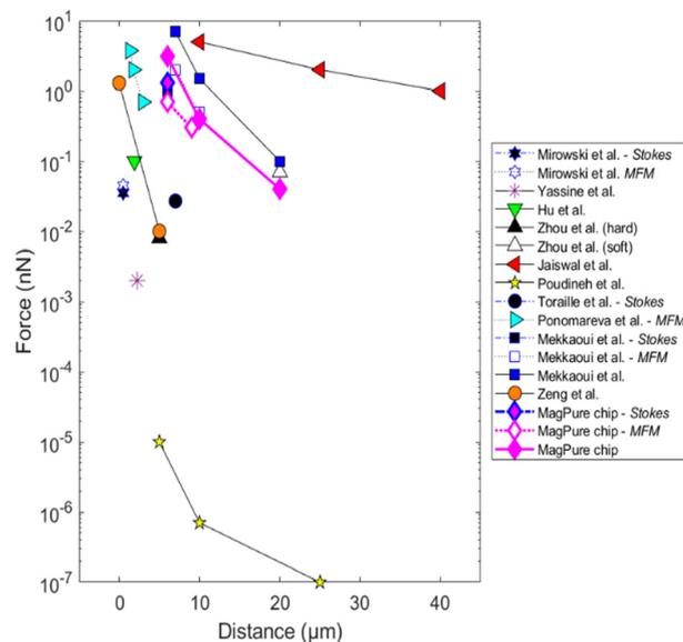
**Fig. 2** Comparison of the magnetic performances of the fabricated composite micro-magnets with other microscale magnetic sources from the literature. The graph represents the forces exerted on the center of the magnetic target as a function of the distance to the micro-source. When not specified, the magnetic force was determined by numerical studies. A description of the magnetic micro-sources and magnetic force measurement methods can be found in Table S3†
