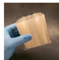
Fig. 1 Development of a mass-producible and deformation-free plastic spiral inertial microfluidic device. (a) A schematic diagram representing the fabrication process of the conventional polydimethylsiloxane (PDMS) spiral device and its stacking process for high-throughput application. (b) A schematic diagram representing the channel deformation in the PDMS spiral device and its effects on the device operation and performance; the color represents the relative channel deformation. (c) A schematic diagram representing the fabrication process of the plastic device and its key advantages; the plastic spiral device was designed by compensating for the channel deformation in the PDMS spiral device.
