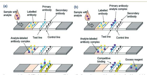
Fig. 1 Schematic representation of LFA detection process utilising antibodies and nanoparticle conjugates for (a) sandwich LFA and (b) competitive LFA.
