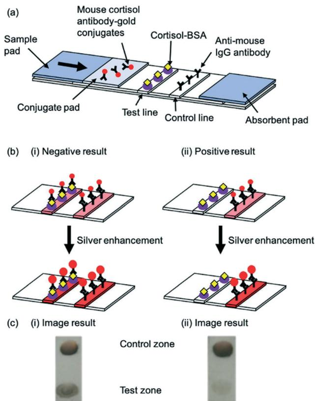
**Fig. 6** Schematic illustration of a competitive salivary cortisol LFA utilising silver enhancement. (a) Schematic of the basic LFA strip and components (b) principle of LFA before and after enhancement for (i) negative result and (ii) positive result (c) image result of the test and control lines for (i) negative result and (ii) positive result. Reproduced with permission.<sup>62</sup> Copyright 2018, PMC.
