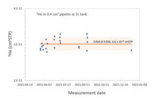
Fig. 5 An example of calibration results of the  ${}^{3}$ He amount in one of the pipettes. Solid line showing the average of all calibration results (n = 23) and shaded band signifying 2 sigma errors are shown.
