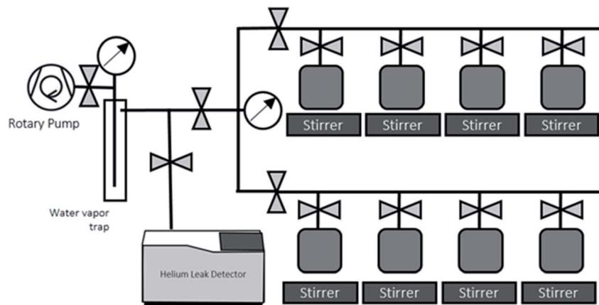
Fig. 3 Water degassing unit for  $^3\text{He}$ -ingrowth analysis.
