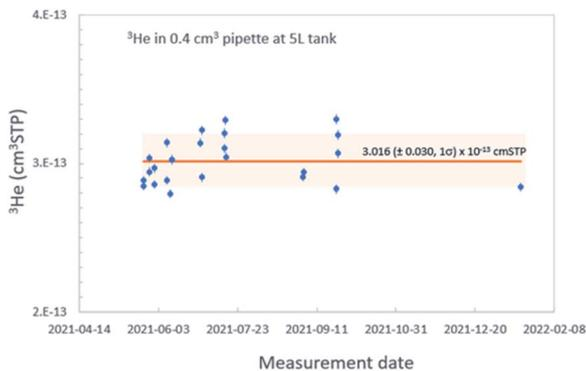
Fig. 5 An example of calibration results of the  $^3\text{He}$  amount in one of the pipettes. Solid line showing the average of all calibration results ( $n = 23$ ) and shaded band signifying 2 sigma errors are shown.
