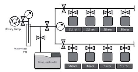
Fig. 3 Water degassing unit for <sup>3</sup>He-ingrowth analysis
