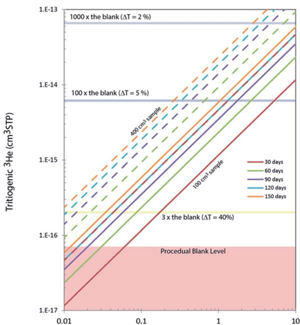
Fig. 6 Tritogenic  $^3\text{He}$  in 100 and 400  $\text{cm}^3$  of water produced in different storage time. A typical level of procedural background of  $^3\text{He}$  in our analytical system is also shown.  $\Delta T$  denotes  $2\sigma$  relative uncertainties expected for given amount of tritogenic  $^3\text{He}$ . Analysis of 0.2 TU samples can be measured with about 5% ( $2\sigma$ ) uncertainties for a 400  $\text{cm}^3$  water sample stored more than 150 days.
