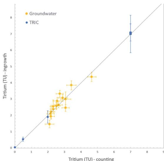
Fig. 7 Comparison of tritium analysis on groundwater samples by decay counting and by the <sup>3</sup>He ingrowth method. A 1 : 1 line is shown for reference. Results of analysis on the TRIC analysis are also shown.
