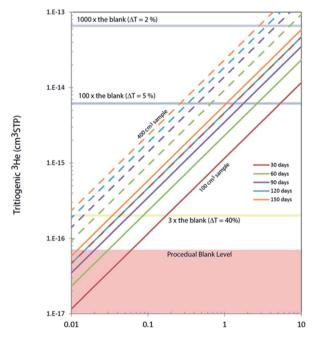
Fig. 6 Tritiogenic  $^3$ He in 100 and 400 cm $^3$  of water produced in different storage time. A typical level of procedural background of  $^3$ He in our analytical system is also shown.  $\Delta T$  denotes  $2\sigma$  relative uncertainties expected for given amount of tritiogenic  $^3$ He. Analysis of 0.2 TU samples can be measured with about 5% ( $2\sigma$ ) uncertainties for a 400 cm $^3$  water sample stored more than 150 days.
