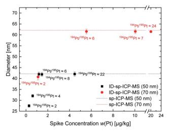
**Fig. 2** Calculated diameters for the platinum nanoparticles (nominal diameter 50 nm and 70 nm). The squares and circles indicate the results obtained by on-line ID-MDG-sp-ICP-ToF-MS for different <sup>194</sup>Pt/<sup>195</sup>Pt isotopic ratios and the dashed lines indicate the results obtained by classical sp-ICP-ToF-MS. The error bars represent the standard deviation of three independent measurements.
