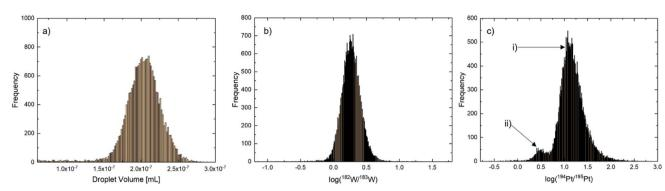
Fig. 1 Volume distribution of the droplets of the MDG (a); isotope ratio distribution of the tungsten (<sup>182</sup>W/<sup>183</sup>W) (b) and platinum (<sup>194</sup>Pt/<sup>195</sup>Pt) without (c, (i)) and with (c, (ii)) platinum nanoparticles (50 nm) present in the droplets.
