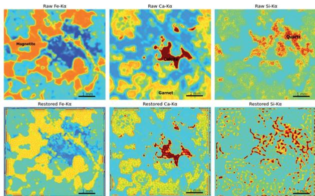
Fig. 9 XRF images of an iron skarn sample.
