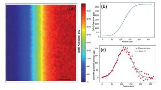
Fig. 4 Knife edge method measurement of the size of the XRF spot. (a) XRF image of the edge of a square on USAF 1951 corresponding to the blue box in Fig. 2(c). (b) XRF intensity distribution crossing the edge. (c) XRF intensity gradient denoting the shape of the XRF spot. The red dots are gradient values of the XRF intensity, and the blue line is the curve fitted by the Gaussian model.
