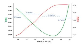
Fig. 8 Image quality (MSE and SSIM) and resolution change with the size of the PSF.
