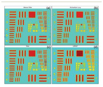
Fig. 5 Results of four image restoration methods: (a) Wiener filter, (b) Richardson–Lucy, (c) fast iterative shrinkage-thresholding algorithm (FISTA), and (d) blind deblurring with L0-regularized intensity and gradient prior (L0RIGP).
