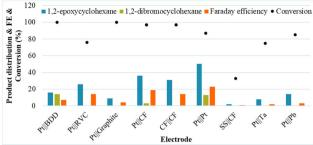
Fig. 1 Product distribution with various electrodes. Reaction conditions: cathode||anode, constant current of 10 mA cm<sup>-2</sup>, 1a (50 mM), NaBr (1.0 eq.), MeCN/H<sub>2</sub>O (4:1, 6 ml), room temperature, 3 h. Yield was determined by GC analysis using octane as the external standard compared with the desired cyclohexene oxide.
