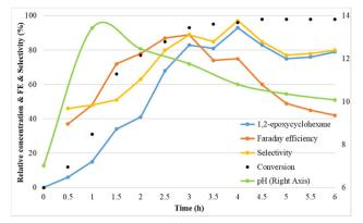
Fig. 4 Reaction conditions: Pt as anode and Pt as cathode, constant current of 7.5 mA cm $^{-2}$ , 1a (75 mM), Et<sub>4</sub>NBF<sub>4</sub> (2 eq.), NaBr (1.5 eq.), MeCN: H<sub>2</sub>O (3: 2, 6 ml), room temperature.
