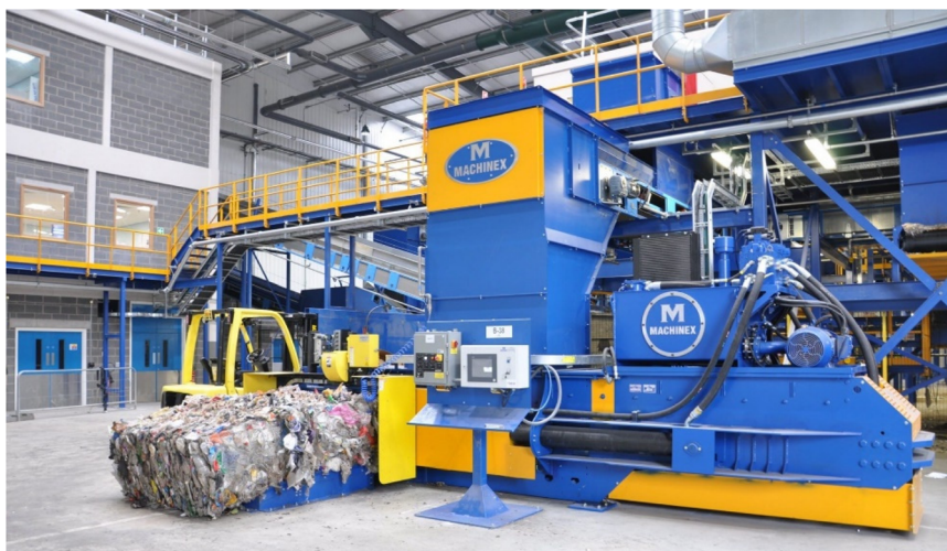
Fig. 11 Two-ram Baler from Machinex Recycling. Reproduced from ref. 104 with permission from Machinex Technologies, copyright 2022.
