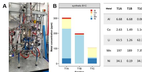
**Fig. 9** Scale-up of Mn removal with synthetic leachates. (A) Semi-pilot reactor vessel (FlexBio, IBIOLC) and (B) Mn recovery (ppm) from a synthetic leachate based on B1C cathode dissolved in 0.5 M H<sub>2</sub>SO<sub>4</sub>.
