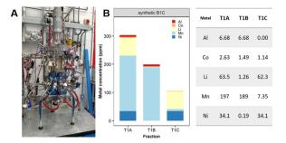
Fig. 9 Scale-up of Mn removal with synthetic leachates. (A) Semi-pilot reactor vessel (FlexBio, IBioIC) and (B) Mn recovery (ppm) from a synthetic leachate based on B1C cathode dissolved in  $0.5 \text{ M H}_2\text{SO}_4$ .
