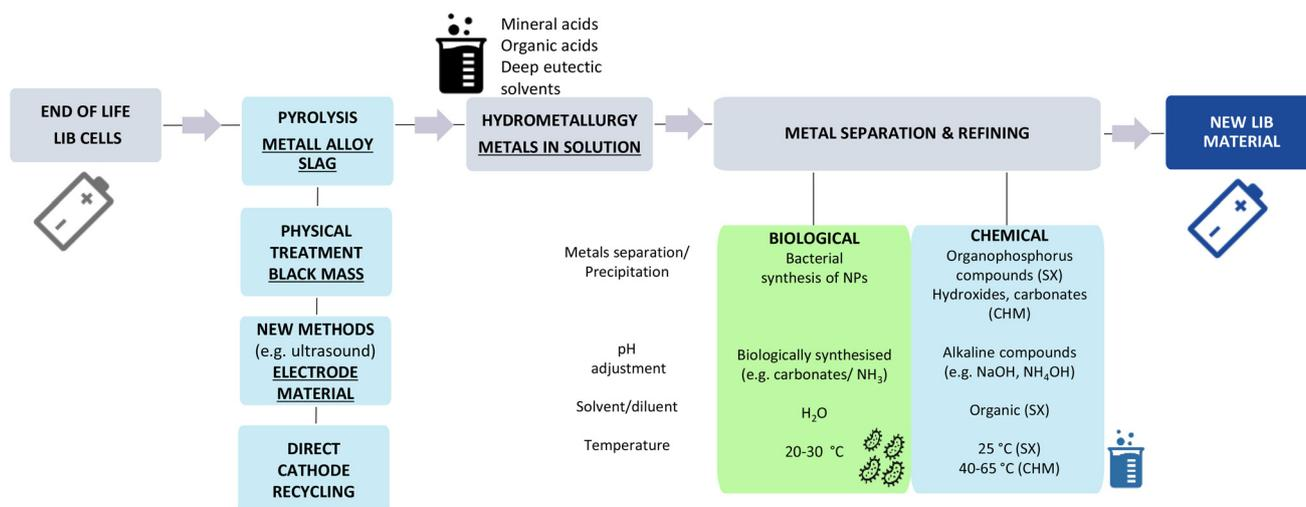
**Scheme 1** Recycling scheme depicting conventional and novel recycling processes for end of life LIB cells and resulting fractions (underlined) containing metals. The reaction conditions of the metal bioseparation process presented in this study (green box) is depicted side by side with conventional chemical separation methods (SX: solvent exchange; CHM: chemical precipitation with *e.g.* hydroxides, carbonates).
