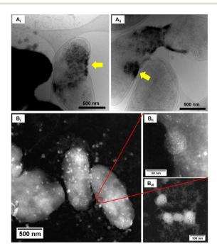
Fig. 5 Characterisation of Co nanoparticles. (A) Cryo-EM images of D. alaskensis G20 incubated for 20 h in Co<sup>2+</sup> 50 ppm, yellow arrows point at high-density areas in the bacterial envelope where Co-based nanoparticles were formed. (B) STEM image of mesoporous nanostructures synthesised on the bacterial envelope of D. alaskensis G20 cells incubated for 20 h in Co<sup>2+</sup> 50 ppm.
