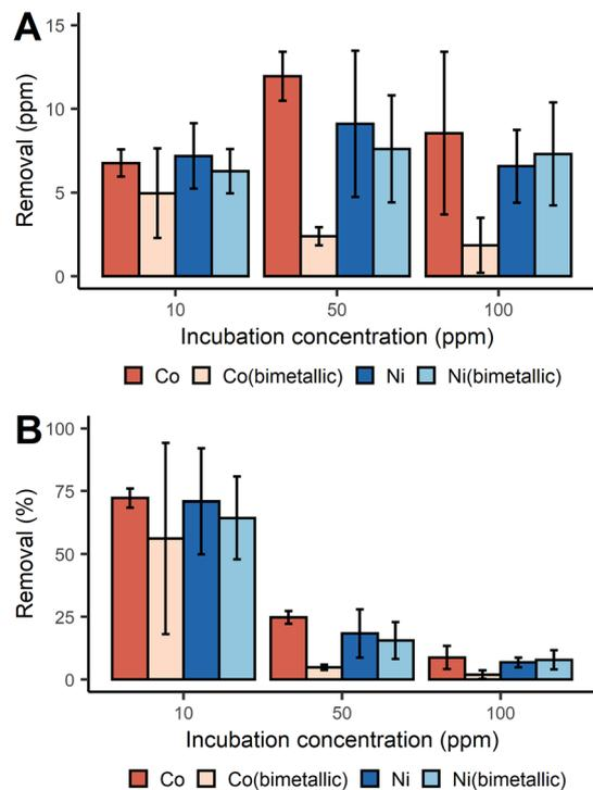
**Fig. 2** Removal of Co<sup>2+</sup> and Ni<sup>2+</sup> with *D. alaskensis* G20 expressed as mean  $\pm$  SD ( $n = 3$ ) measured as (A) ppm and (B) percent.
