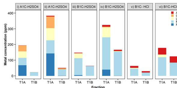
Fig. 7 Bioprecipitation of metals contained in vehicular LIBs using *S. oneidensis* MR-1. Selected leachates: cathode A1C at 50 °C in 0.1 M H<sub>2</sub>SO<sub>4</sub> for (i) 5 min and (ii) 30 min; cathode B1C at 50 °C in 0.1 M H<sub>2</sub>SO<sub>4</sub> for (iii) 5 min and (iv) 30 min; cathode B1C at 20 °C in 0.1 M HCl for (v) 5 min and (vi) 300 min. Metal concentration in the raw leachate (T1A) and metal removal/precipitated (T1B) expressed as the mean ( $n = 3$  biological replicates).
