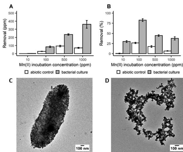
**Fig. 1** Removal of dissolved Mn<sup>2+</sup> expressed as mean ± SD (*n* = 3) measured as (A) ppm and (B) percent with cell cultures of *S. oneidensis* MR-1 and abiotic control. TEM images of nanoparticles produced by *S. oneidensis* MR-1 incubated with 1000 ppm of Mn<sup>2+</sup> (C) coating the bacterial cells and (D) detached from bacterial biomass.
