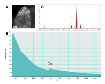
**Fig. 4** Characterisation of Co nanoparticles by STEM, EDXS and EELS. (A) STEM image, (B) EELS and (C) EDXS spectra taken from the spot highlighted with red square on image (A), on the surface of D. alaskensis G20 incubated for 20 h in  $Co^{2+}$  10 ppm, and re-suspended at a final concentration of ethanol 50% v/v. Cu peaks in the EDXS are associated to the TEM grid.
