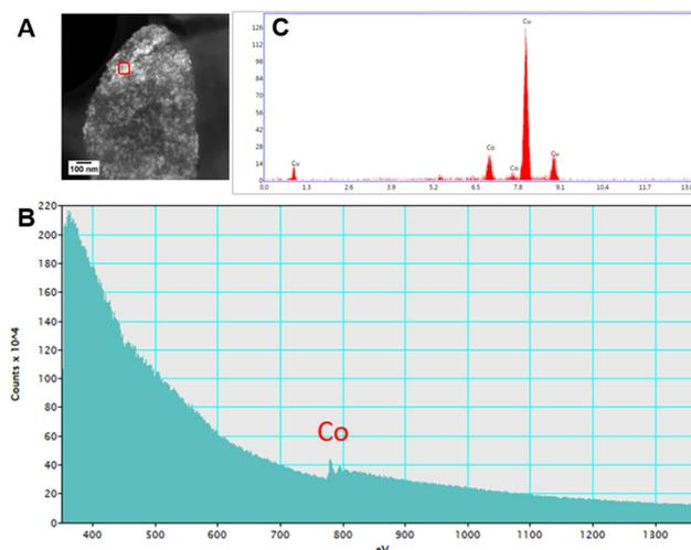
**Fig. 4** Characterisation of Co nanoparticles by STEM, EDXS and EELS. (A) STEM image, (B) EELS and (C) EDXS spectra taken from the spot high-lighted with red square in image (A), on the surface of *D. alaskensis* G20 incubated for 20 h in Co<sup>2+</sup> 10 ppm, and re-suspended at a final concentration of ethanol 50% v/v. Cu peaks in the EDXS are associated to the TEM grid.
