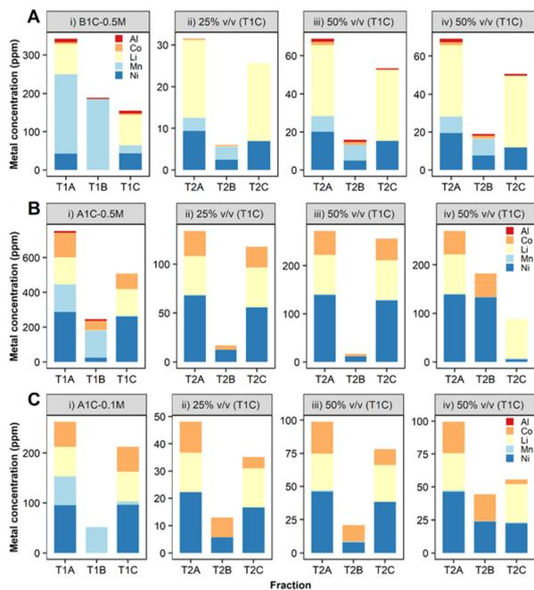
**Fig. 8** Bio-separation of metals contained in leachates prepared with (A) B1C 0.5 M H<sub>2</sub>SO<sub>4</sub> (B) A1C 0.5 M (C) A1C 0.1 M H<sub>2</sub>SO<sub>4</sub>. Metal concentration expressed as the mean ( $n = 3$  biological replicates) associated to different stages of (i) T1 and T2 (ii and iii) cell-only treatment (thoroughly washed bacterial cells in MOPS buffer) and (iv) whole bacterial cell culture.
