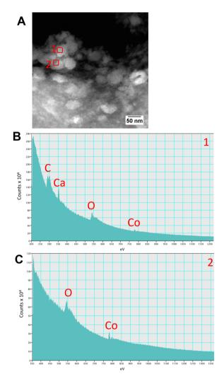
Fig. 6 Characterisation of the mesoporous nanostructures using (A) STEM and (B and C) EELS spectra obtained from regions (A) 1 and 2 highlighted with red squares.
