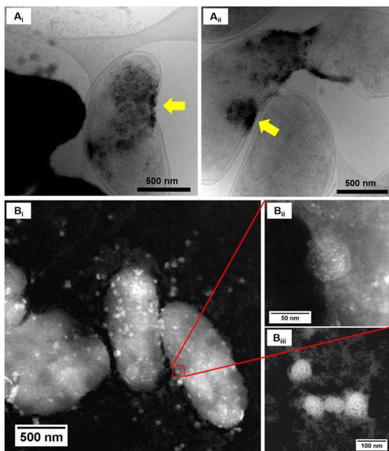
**Fig. 5** Characterisation of Co nanoparticles. (A) Cryo-EM images of *D. alaskensis* G20 incubated for 20 h in  $\text{Co}^{2+}$  50 ppm, yellow arrows point at high-density areas in the bacterial envelope where Co-based nanoparticles were formed. (B) STEM image of mesoporous nanostructures synthesised on the bacterial envelope of *D. alaskensis* G20 cells incubated for 20 h in  $\text{Co}^{2+}$  50 ppm.
