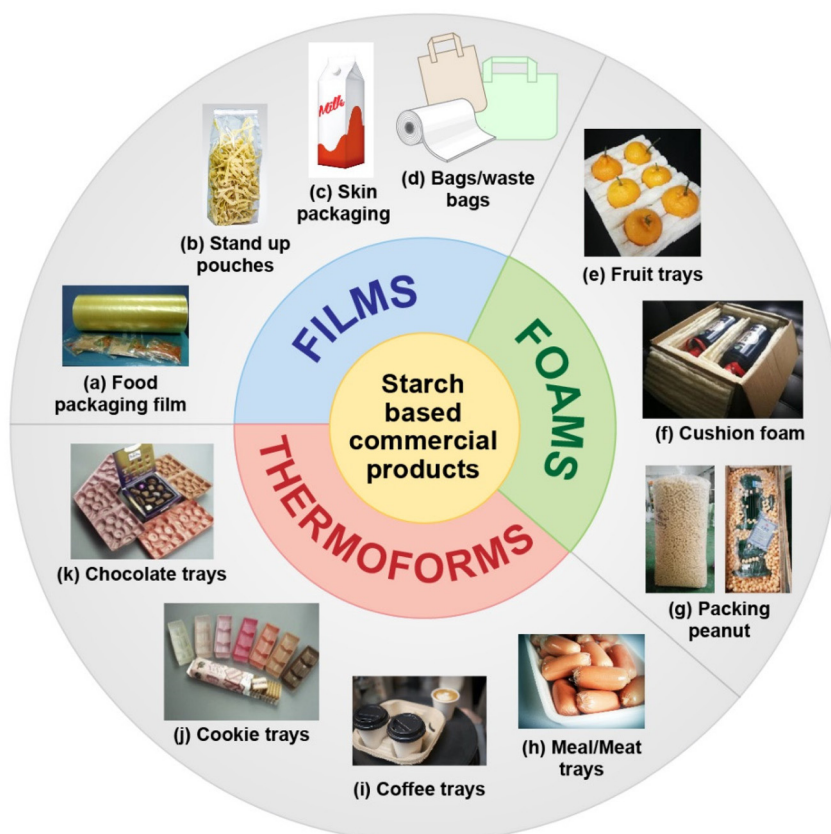
Fig. 15 Real-life applications of starch-based materials classified as: (i) films which includes (a) food packaging films, (b) stand-up pouches, (c) skin packaging and (d) bags/waste bags; (ii) foams which includes (e) fruit trays, (f) cushion foam, (g) packing peanuts; (iii) thermoforms which includes (h) meal/meat trays, (i) coffee trays, (j) cookies trays, (k) chocolate trays. ((a) (Reproduced from ref. 255 with permission from Elsevier, copyright 2019), (b) and (h) pixabay free images, pictures (e), (f), (g), (j), (k) have been taken from open access article under a Creative Commons licence attribution-non-commercial-no derivatives 4.0 international ref. 246, picture (i) from "Icons" of Microsoft office.)
