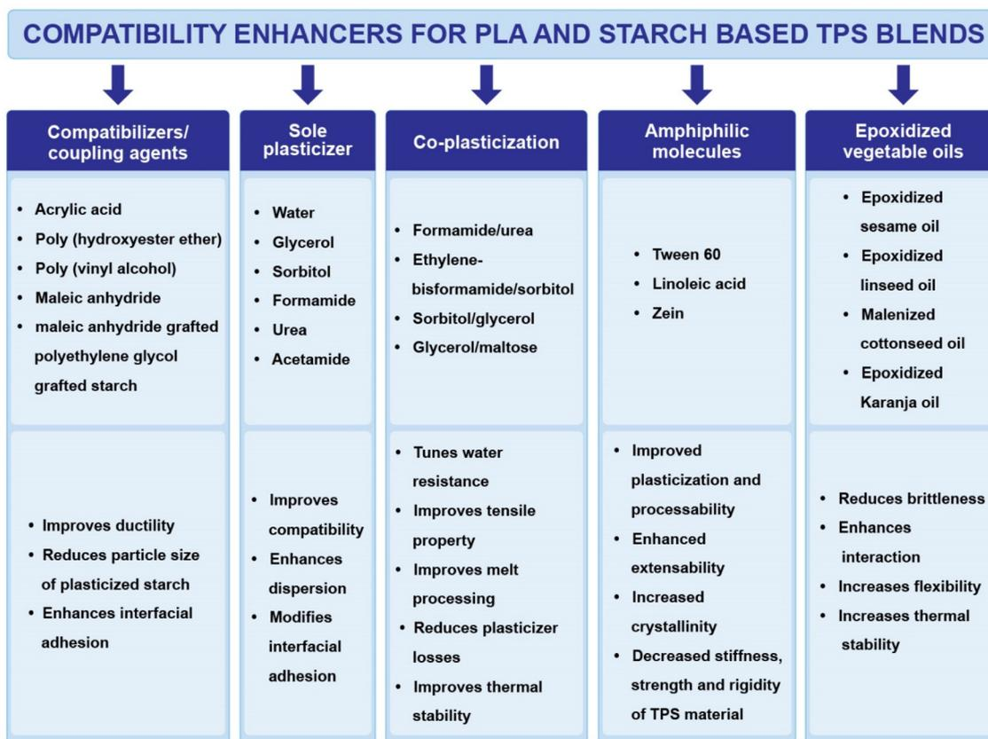
**Fig. 13** Shows the compilation of different strategies and resultant properties obtained on use of compatibilizers/coupling agents, individual (sole) plasticizer, co-plasticization, amphiphilic molecules and epoxidized oils in PLA/starch-based blends systems (drawn by author).
