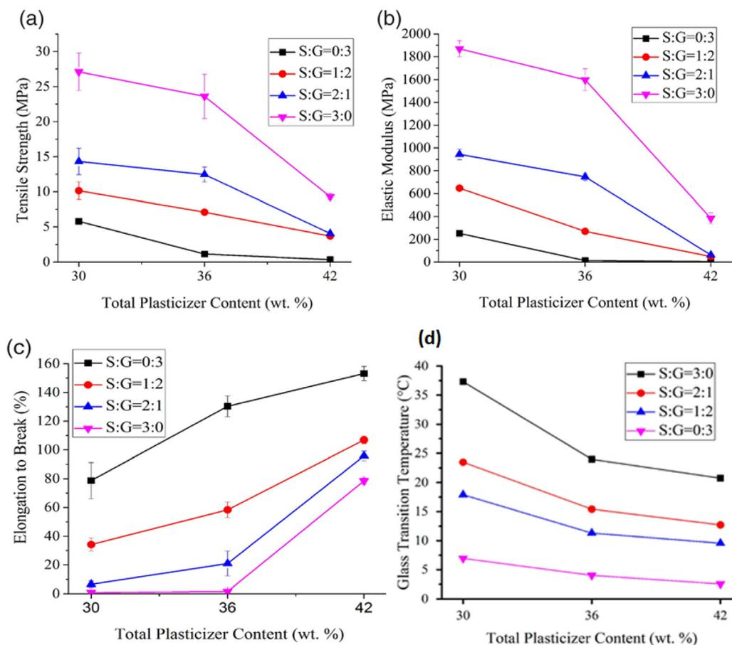
Fig. 5 The variation in thermomechanical properties of sorbitol/glycerol co-plasticized starch at different weight ratio and total plasticizer content. (a) Tensile strength (b) elastic modulus (c) elongation at break and (d) glass transition temperature. Reproduced from ref. 132 with permission from John Wiley and Sons, copyright 2017.
