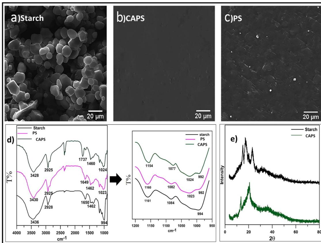
Fig. 7 (a) SEM micrograph of starch, (b) SEM micrograph of CAPS, (c) SEM micrograph of PS, (d) FTIR spectroscopy of starch, CAPS and PS, (e) XRD of starch and CAPS. Reproduced from ref. 63 with permission from Elsevier, copyright 2019.
