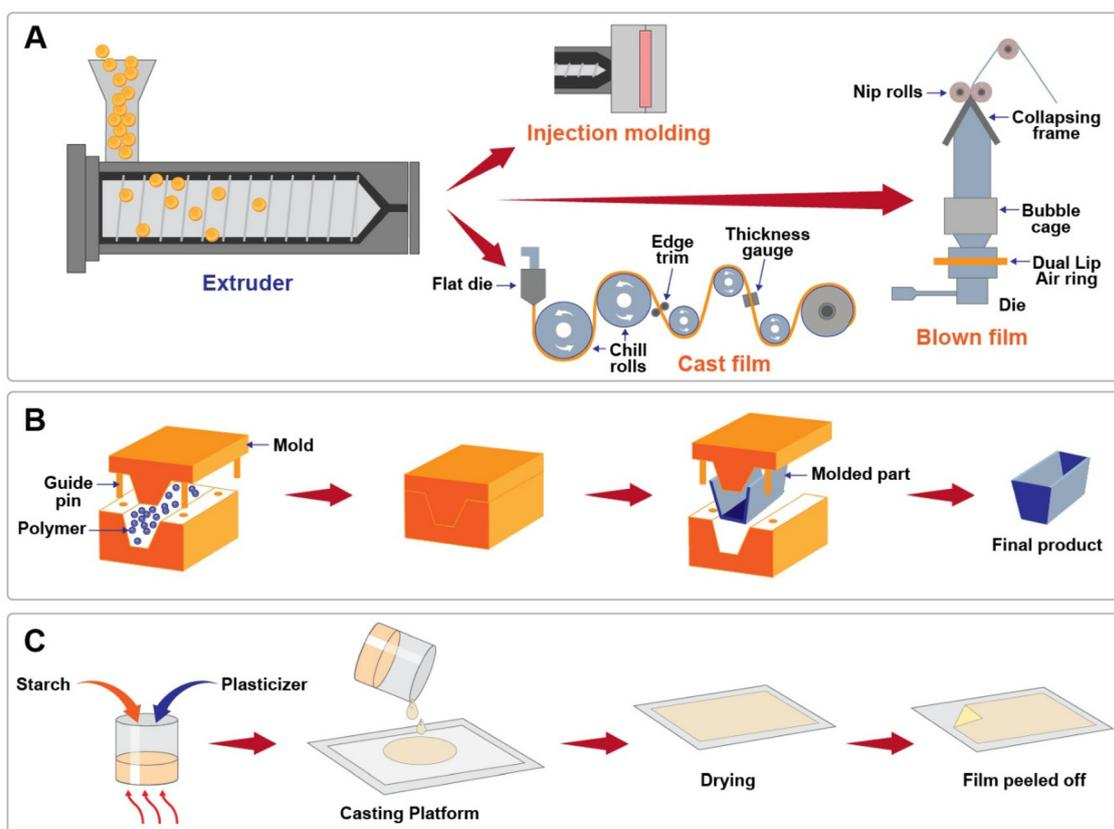
**Fig. 8** Processing techniques (A) extrusion technique (B) compression moulding and (C) solution casting followed by injection for rigid-type applications and blown film or cast film for flexible packaging type applications (drawn by author).
