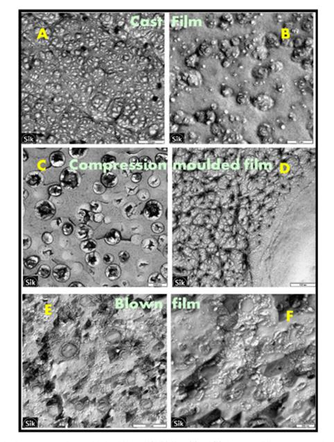
Fig. 9 TEM micrograph of cast, compression moulded and blown HONPS films. (A) and (B) shows two different structures in cast HONPS with scale bars 100 nm, (C) and (D) shows compression moulded (HONPS) with scale bars 2000 and 100 nm, (E) and (F) shows blown HONPS films with scale bars of 1000 nm and 200 nm respectively. Reproduced from ref. 138 with permission from Elsevier, copyright 2008.
