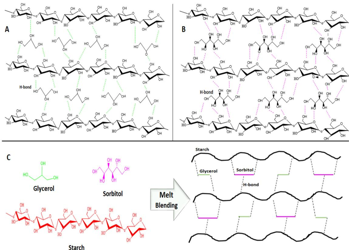
**Fig. 6** Shows the schematic representation of hydrogen bonds formed during the plasticization of starch with (A) glycerol, (B) sorbitol and (C) glycerol/sorbitol after melt blending (molecular structures drawn by author using ChemDraw).<sup>132</sup>
