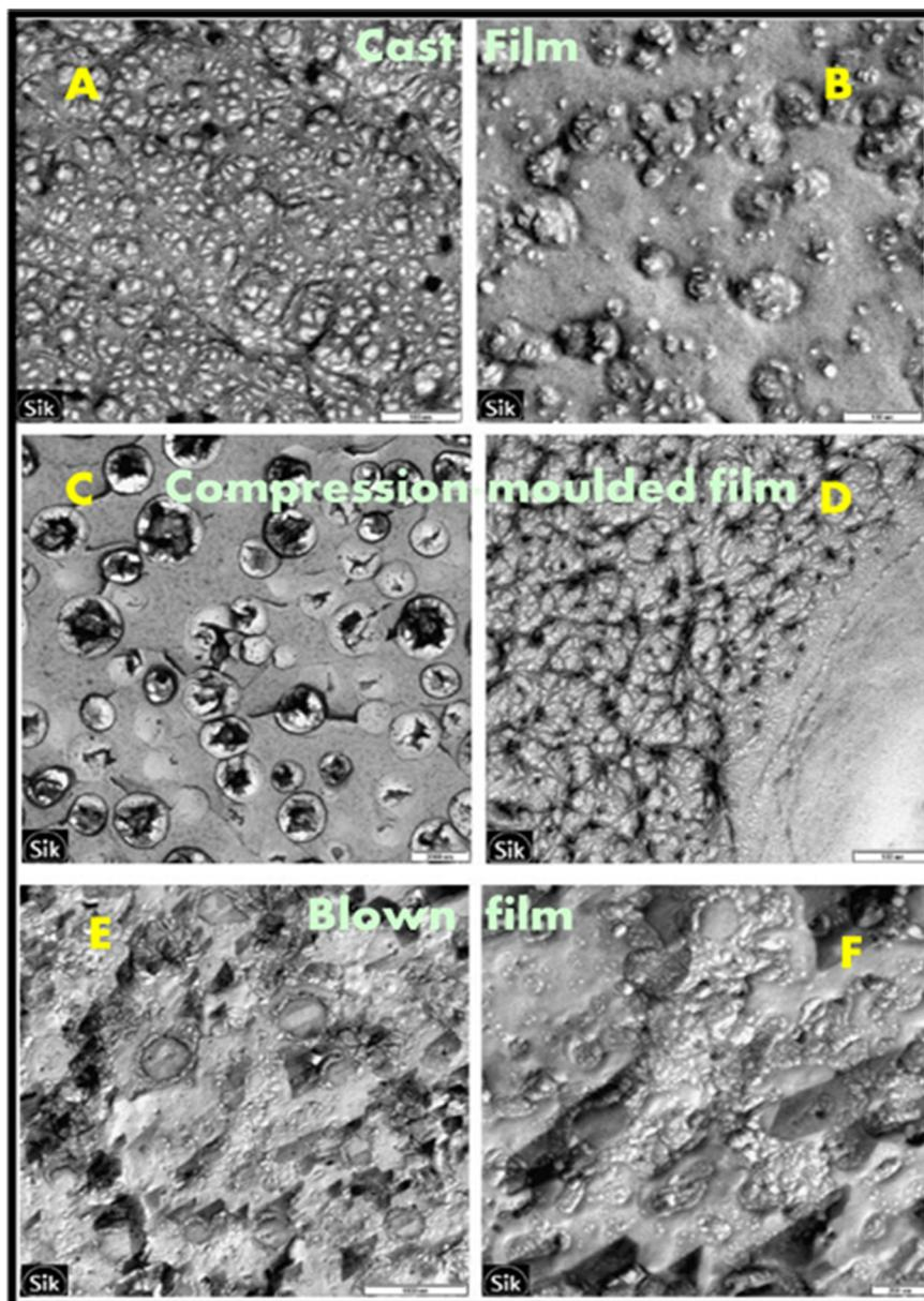
**Fig. 9** TEM micrograph of cast, compression moulded and blown HONPS films. (A) and (B) shows two different structures in cast HONPS with scale bars 100 nm, (C) and (D) shows compression moulded (HONPS) with scale bars 2000 and 100 nm, (E) and (F) shows blown HONPS films with scale bars of 1000 nm and 200 nm respectively. Reproduced from ref. 138 with permission from Elsevier, copyright 2008.
