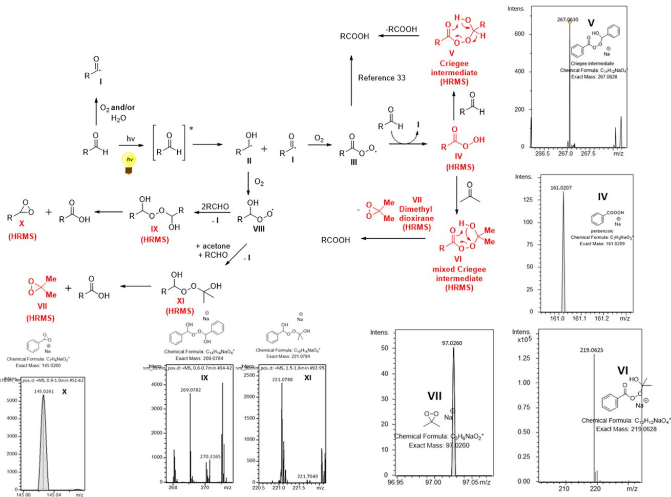
**Scheme 3** Proposed mechanism for the oxidation of aldehydes to carboxylic acids in acetone/water and selected HRMS spectra of the oxidation of benzaldehyde, verifying the generation of peracid IV, Criegee intermediate V, mixed Criegee intermediate with acetone VI, dimethyl dioxirane VII and intermediates IX, X and XI.
