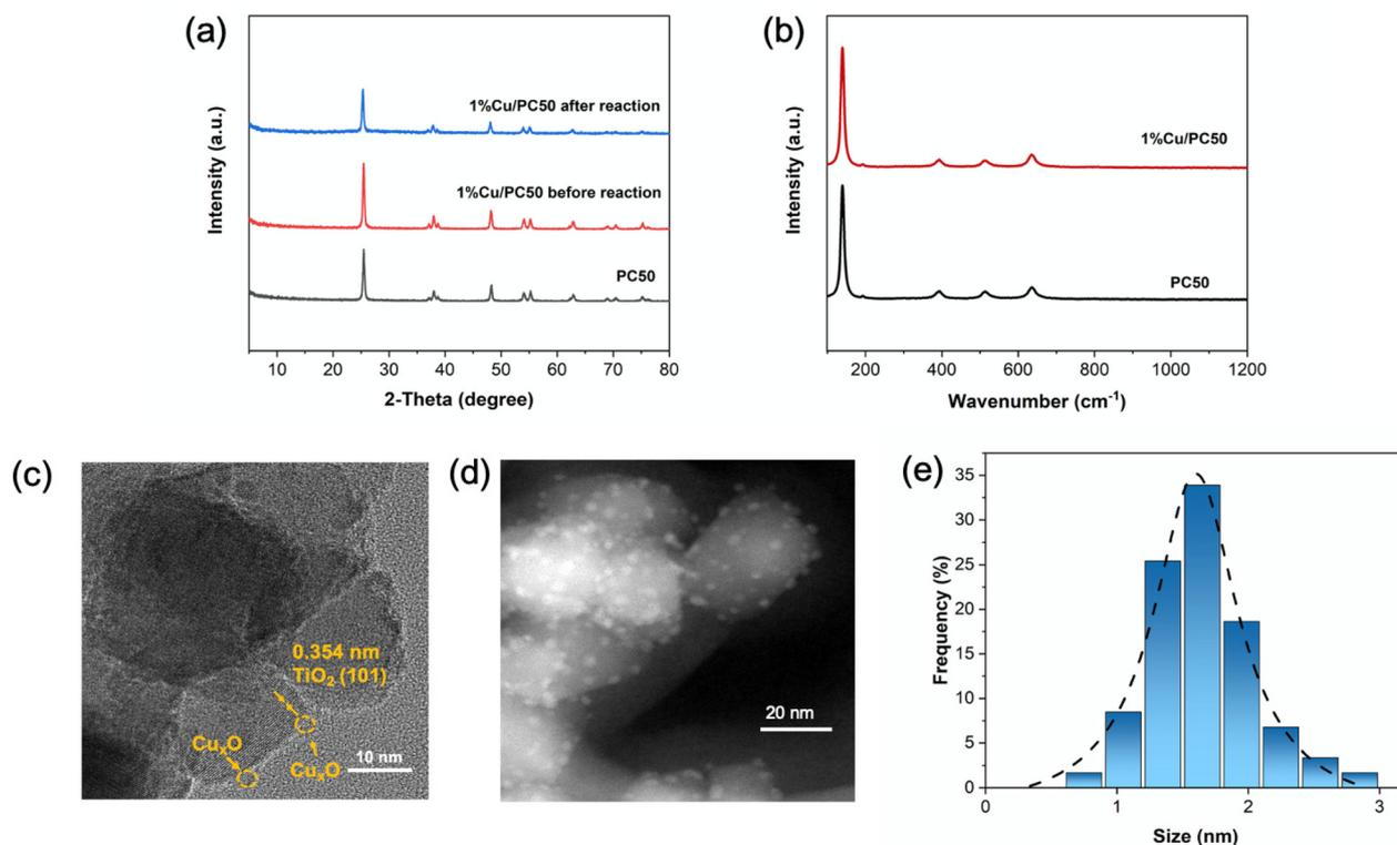
**Fig. 4** (a) PXRD and (b) Raman spectra of 1% Cu/PC50 and PC50. (c) HR-TEM and (d) HAADF images of 1% Cu/PC50 in which highly dispersed  $Cu_xO$  particles are very clear. (e) The size distribution of  $Cu_xO$  nanoparticles on a PC50 surface obtained by counting of 60 particles from the HAADF picture of 4d.
