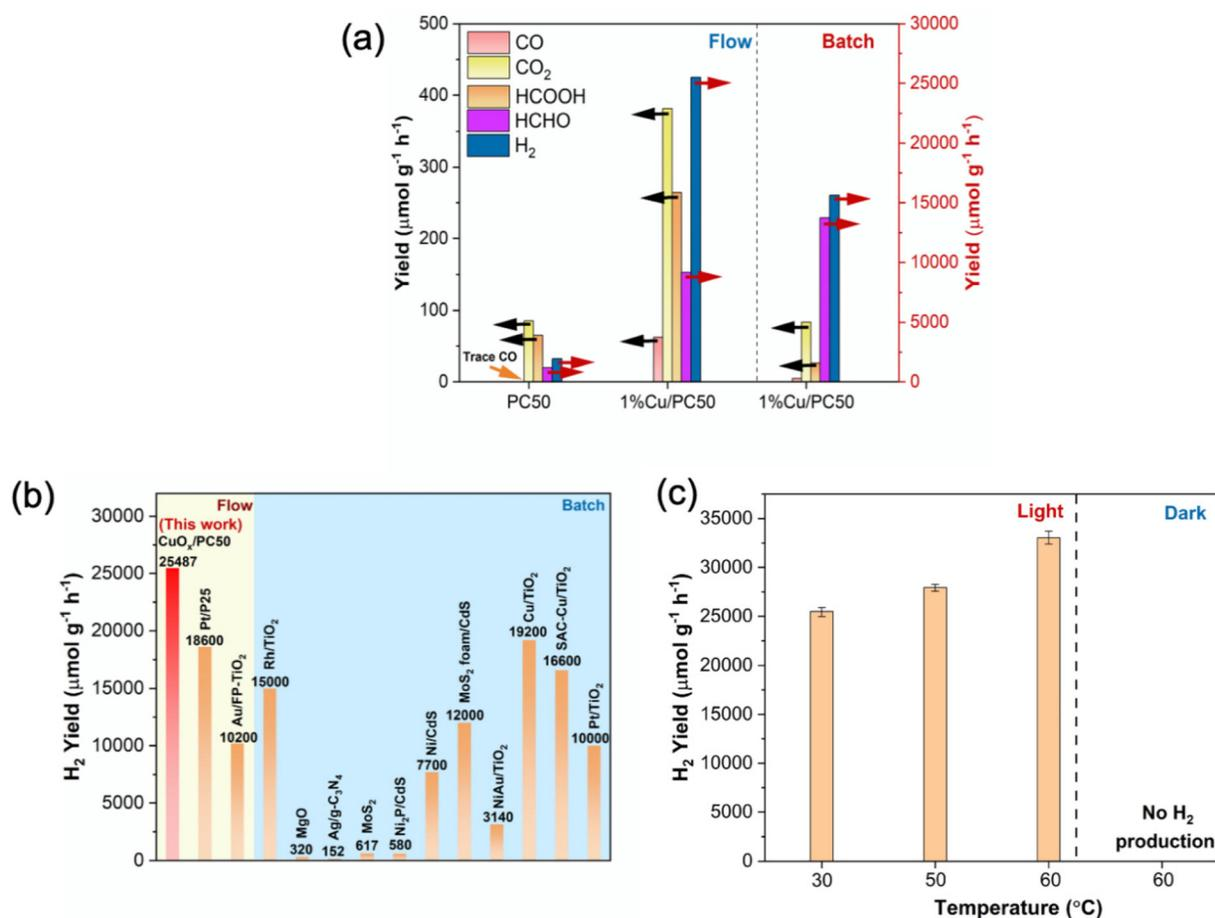
**Fig. 3** (a) The yield of  $\text{H}_2$  and oxidation products by a flow (left panel) and a batch reactor (right panel). (b) Comparison of the  $\text{H}_2$  yield over different photocatalysts for  $\text{H}_2$  production from methanol reported to date. All results were achieved at room temperature. (c)  $\text{H}_2$  yield from a methanol and water mixture by photocatalysis over 1% Cu/PC50 at different temperatures.
