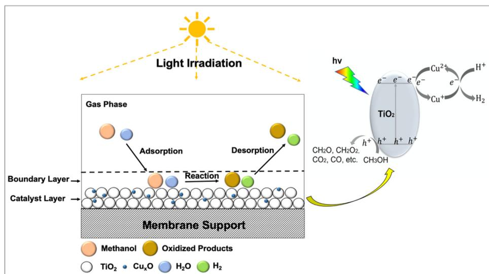
**Scheme 1** Proposed schematic illustration of photocatalytic methanol dehydrogenation and reforming on 1% Cu/PC50 in the flow membrane reactor.
