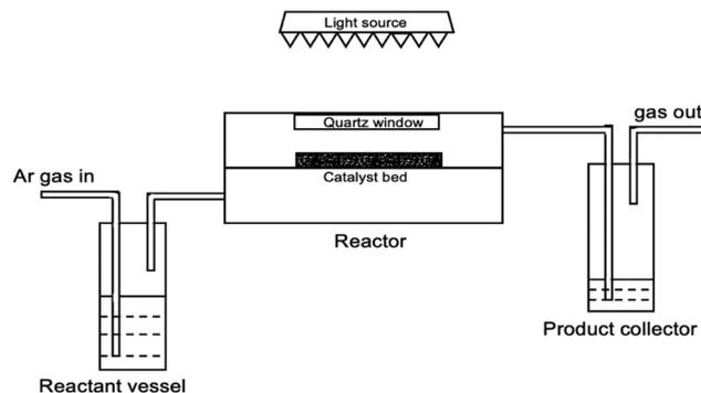
Fig. 1 The diagram of a flow membrane reactor for photocatalytic methanol dehydrogenation and reforming.
