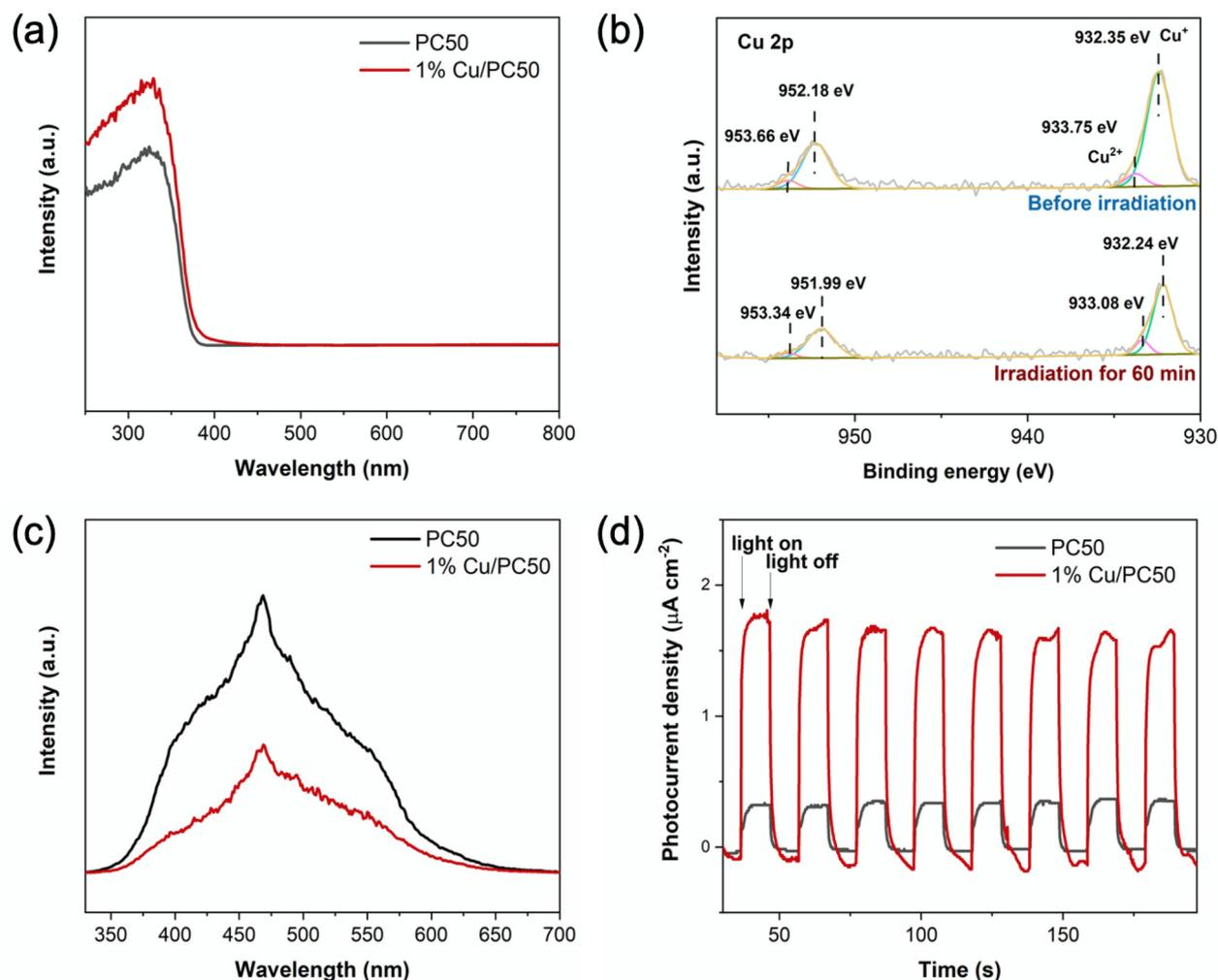
Fig. 5 (a) UV-Vis-DRS spectra of PC50 and 1% Cu/PC50. (b) *In situ* XPS spectra of Cu 2p on 1% Cu/PC50 in the dark and under light illumination. (c) PL spectra of PC50 and 1% Cu/PC50. (d) Photocurrent response curve of 1% Cu/PC50 and PC50 in 0.1 M Na<sub>2</sub>SO<sub>4</sub> with 10 vol% methanol and 0.1 V bias versus Ag/AgCl.
