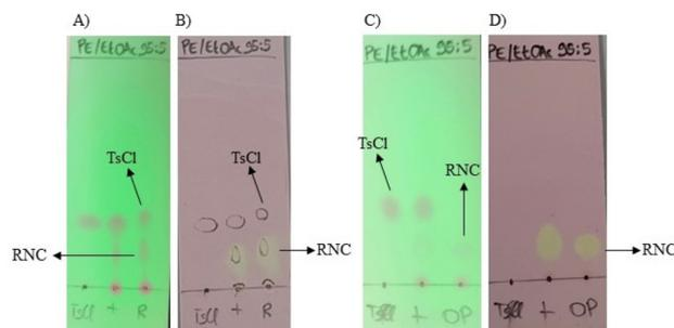
**Fig. 2** (A) TLC under UV before the work up; (B) TLC using 0.5% of py-tetrazine in methanol as staining reagent, before the work up; (C) TLC under UV after the work up; (D) TLC using 0.5% of py-tetrazine in methanol as staining reagent, after the work up. (A) and (B) from left to right: *p*-TsCl, cospot, reaction mixture (C) and (D) from left to right: *p*-TsCl, cospot, organic phase.
