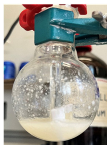
Fig. 5 Synthesis of isocyanide 14 in a 10 mmol scale using a mechanical stirrer.
