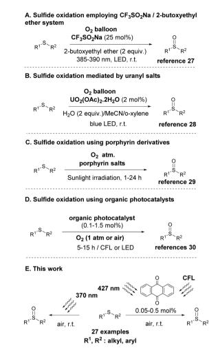
Scheme 2 Photochemical aerobic oxidation of sulfides.
