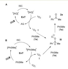
**Scheme 6** Proposed mechanistic pathways for the photochemical aerobic oxidation of thioanisole (1a).
