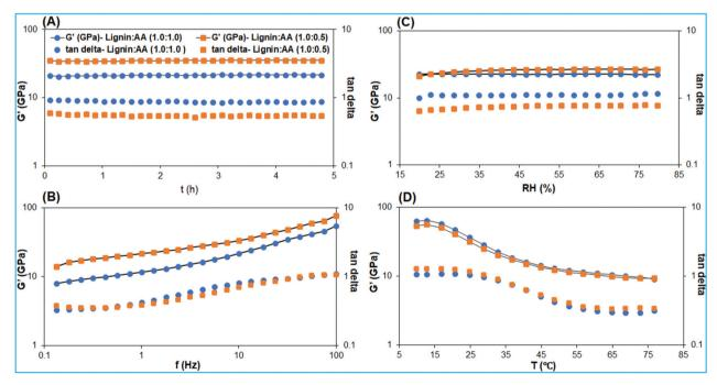
Fig. 4 Mechanical analysis of lignin-based universal adhesive. DMTA for storage modulus (G') of adhesive (with lignin: AA ratios of 1.0:1.0 and 1.0:0.5, wt/wt). (A) Time sweep at 25 °C and 30% RH with a frequency of 10 Hz, (B) frequency sweep at 25 °C and 30% RH, (C) relative humidity (RH) sweep at 25 °C with a frequency of 10 Hz, and (D) temperature sweep at 30% RH with a frequency of 10 Hz and temperature increase rate of 2 K  $min^{-1}$ .
