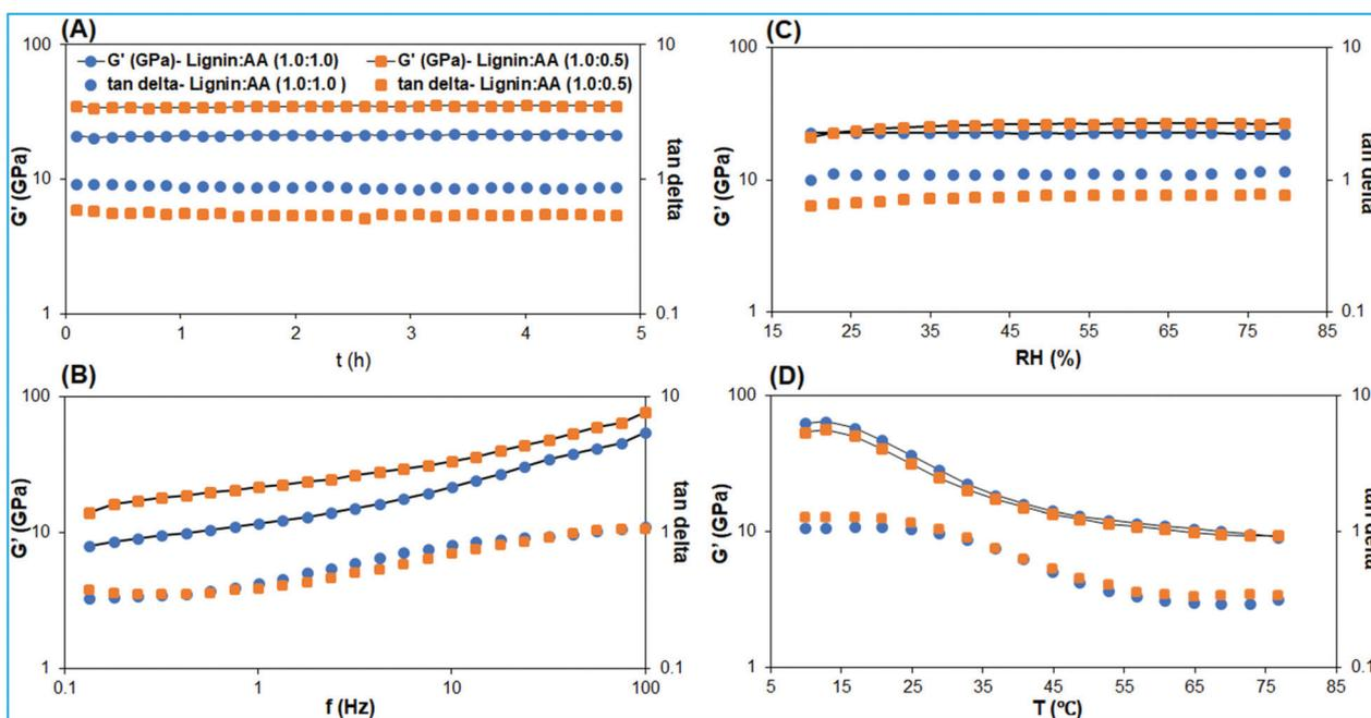
**Fig. 4** Mechanical analysis of lignin-based universal adhesive. DMTA for storage modulus ( $G'$ ) of adhesive (with lignin : AA ratios of 1.0 : 1.0 and 1.0 : 0.5, wt/wt). (A) Time sweep at 25 °C and 30% RH with a frequency of 10 Hz, (B) frequency sweep at 25 °C and 30% RH, (C) relative humidity (RH) sweep at 25 °C with a frequency of 10 Hz, and (D) temperature sweep at 30% RH with a frequency of 10 Hz and temperature increase rate of 2 K  $\text{min}^{-1}$ .
