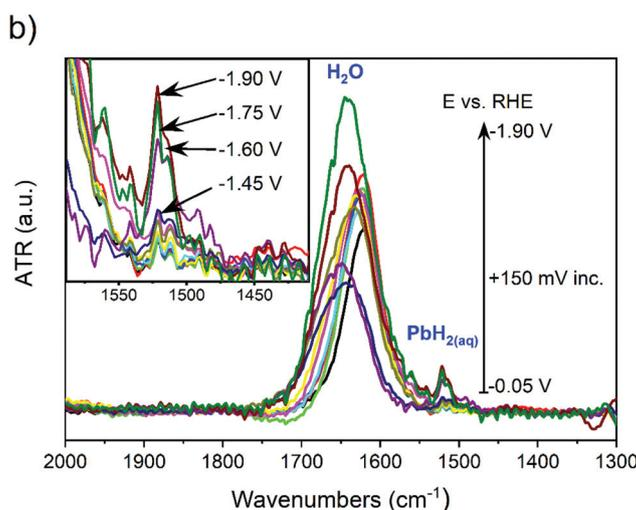
**Fig. 2** (b) *In situ* ATR-FTIR spectra for Pb film polarized at different potentials from –0.05 V to –1.90 V vs. RHE, with steps of 150 mV, in 0.1 M KHCO<sub>3</sub> + 0.1 M KClO<sub>4</sub> at 20 °C.
