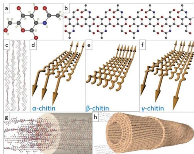
**Fig. 1** The structure and configuration of chitin. (a and b) Ball-and-stick model of the dGlcNAc monomer, where red is oxygen, blue is nitrogen, and gray is carbon atom; (c) schematic diagram of chitin molecular chain arrangement; (d–f) schematic diagrams of the molecular chain orientations in the polymorphic configurations of different types of chitin; (g and h) molecular chain packaging diagram and nanofiber packaging diagram in chitin nanofibers.<sup>54</sup> Copyright 2021 Elsevier Ltd.
