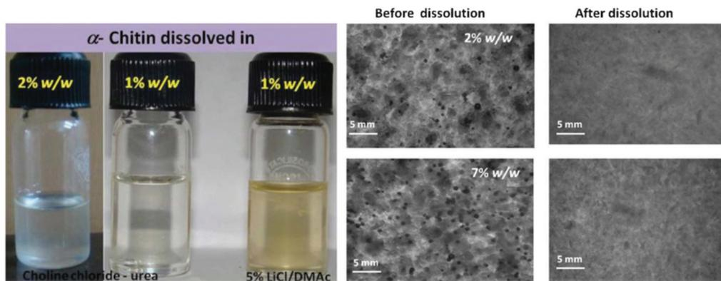
**Fig. 2** (a) Optical photographs of  $\alpha$ -chitin (2% w/w) solubilized in choline chloride/urea DES and 5% LiCl–*N,N*-dimethylacetamide; (b) phase contrast microscopic photograph (1006) of  $\alpha$ -chitin (2% and 7% w/w) in choline chloride–thiourea 1:2 before and after dissolution (ultrasonication assisted heating).<sup>62</sup> Copyright 2013 Royal Society of Chemistry.
