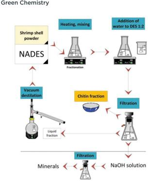
Fig. 5 Sustainable process for chitin and minerals fractionation from shrimp shell by NADES.<sup>65</sup> Copyright 2020 De Gruyter.
