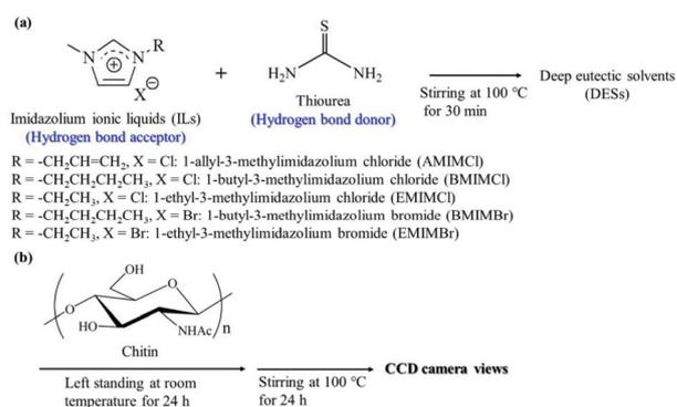
**Fig. 3** (a) Preparation of DESs and (b) dissolution experiment procedure of chitin in DESs.<sup>63</sup> Copyright 2019 Multidisciplinary Digital Publishing Institute.
