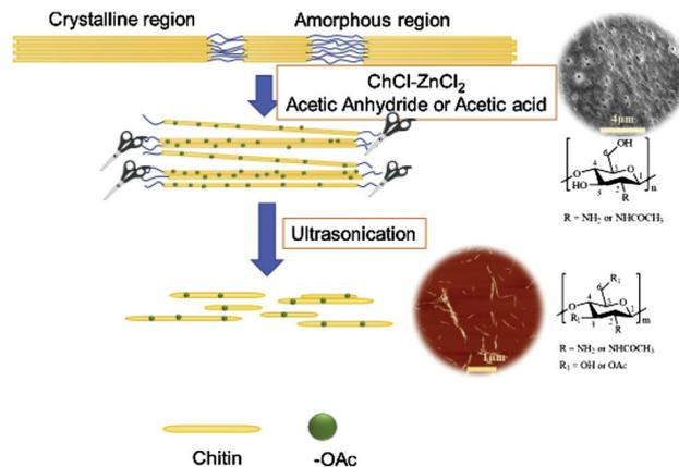
Fig. 6 Schematic diagram of the one-step manufacturing of nanocrystals (CNC).<sup>73</sup> Copyright 2019 Elsevier Ltd.
