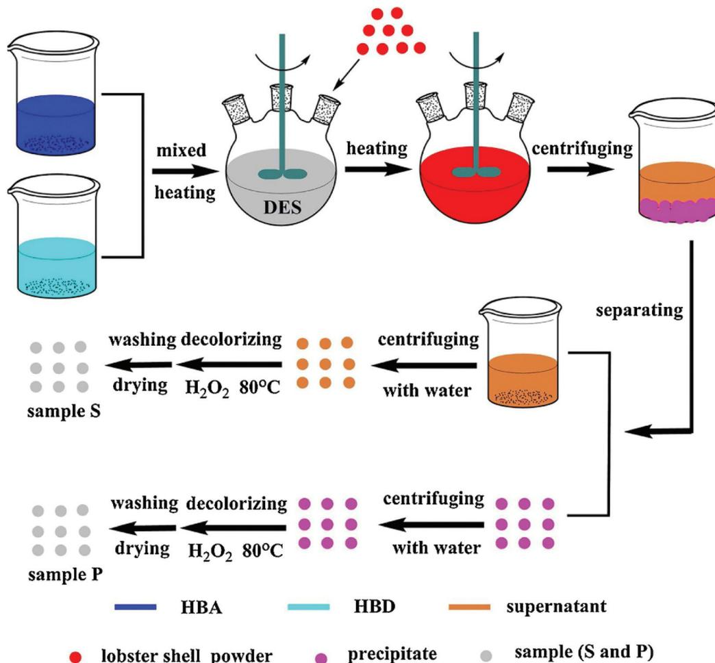
Fig. 4 Schematic diagram of the DES extraction process.<sup>64</sup> Copyright 2017 Elsevier Ltd.
