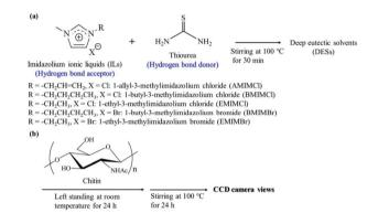
**Fig. 3** (a) Preparation of DESs and (b) dissolution experiment procedure of chitin in DESs.<sup>63</sup> Copyright 2019 Multidisciplinary Digital Publishing Institute.
