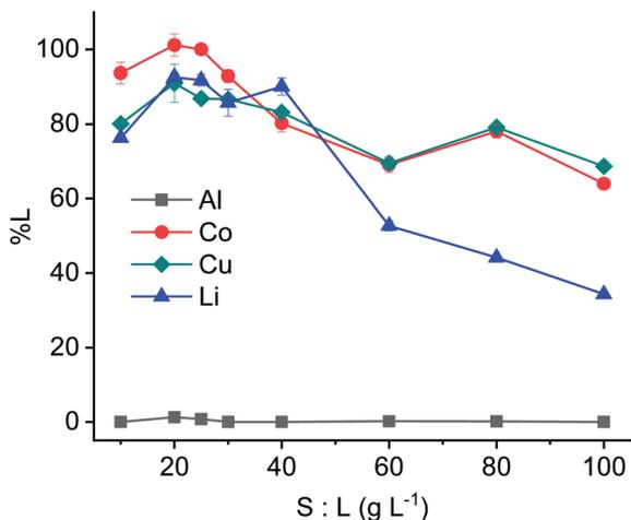
Fig. 3 Percentage leaching by 75 vol% (diluted in an aliphatic diluent) D2EHPA at different S : L ratios. Leaching parameters: 80 °C, 8 hours, 600 rpm. Al : LiCoO<sub>2</sub> = 12 wt%, Cu : LiCoO<sub>2</sub> = 24 wt%.
