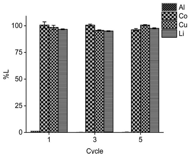
**Fig. 14** Leaching efficiencies of 75 vol% (diluted in an aliphatic diluent) D2EHPA after several cycles. The loaded D2EHPA phase after each cycle was stripped by 1.15 mol L<sup>-1</sup> sulphuric acid at  $V_o : V_a = 2$ , room temperature for 20 minutes at 1750 rpm. The leaching at each cycle was performed at: 80 °C, 6 hours, 25 g L<sup>-1</sup>, 600 rpm. Al : LiCoO<sub>2</sub> = 12 wt%, Cu : LiCoO<sub>2</sub> = 24 wt%.
