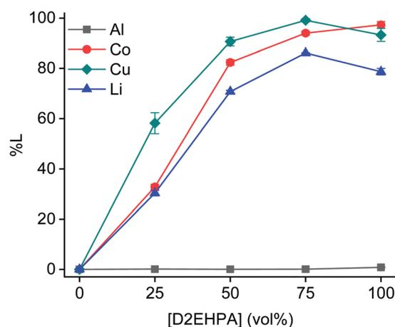
Fig. 2 Percentage leaching by different concentrations of D2EHPA diluted in an aliphatic diluent. Leaching parameters: 80 °C, 8 hours, S:L = 20 g L<sup>-1</sup>, 600 rpm. Al:LiCoO<sub>2</sub> = 12 wt%, Cu:LiCoO<sub>2</sub> = 24 wt%.
