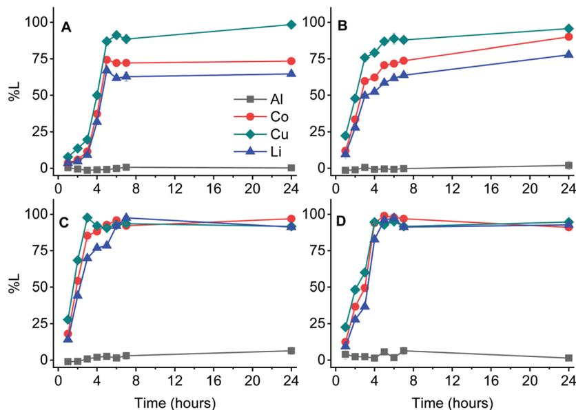
Fig. 4 The percentage leaching during time by 75 vol% (diluted in an aliphatic diluent) D2EHPA at 40 °C (A), 60 °C (B), 80 °C (C) and 100 °C (D). Leaching parameters: 25 g L<sup>-1</sup>, 600 rpm. Al : LiCoO<sub>2</sub> = 12 wt%, Cu : LiCoO<sub>2</sub> = 24 wt%.
