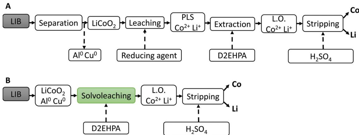
Fig. 16 Summarizing comparison of two processes to recover cobalt from spent LIBs. A conventional hydrometallurgical process above (A) and our proposed solvometallurgical process below (B).
