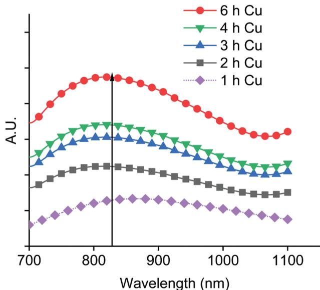
**Fig. 9** UV-VIS absorption spectra of copper complexes with D2EHPA during the leaching of LCO by 75 vol% (diluted in an aliphatic diluent) D2EHPA in presence of Al and Cu, at different time intervals. Leaching parameters: 80 °C, 25 g L<sup>-1</sup>, 600 rpm. Al : LiCoO<sub>2</sub> = 12 wt%, Cu : LiCoO<sub>2</sub> = 24 wt%.
