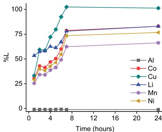
**Fig. 15** The percentage leaching of NMC material during time by 75 vol% (diluted in an aliphatic diluent) leaching parameters: 80 °C, 25 g L<sup>-1</sup>, 600 rpm. Al : NMC = 12 wt%, Cu : NMC = 24 wt%.
