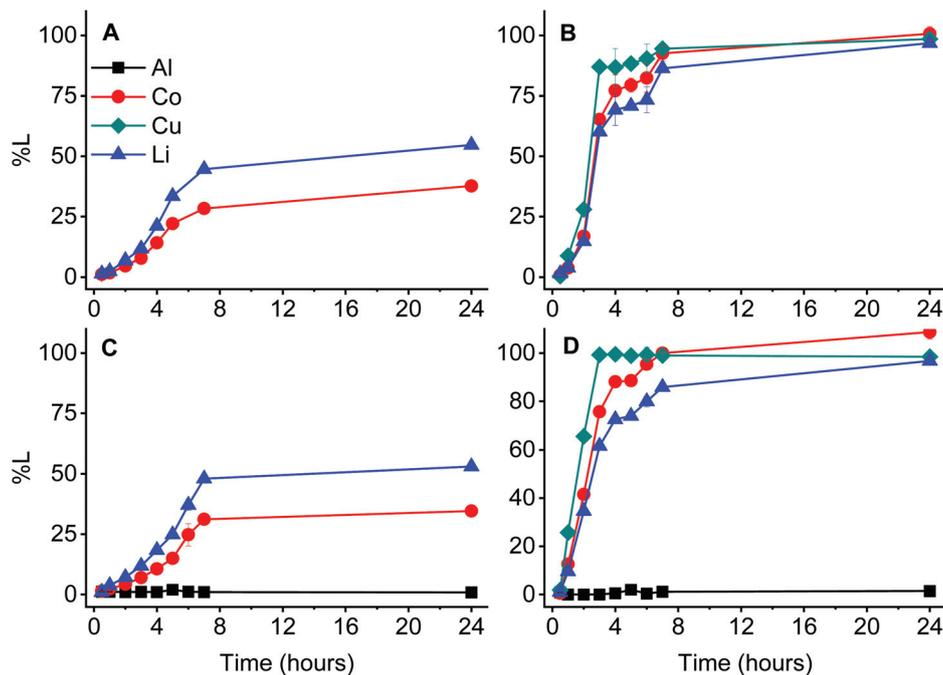
Fig. 5 Leaching efficiencies by 75 vol% (diluted in an aliphatic diluent) D2EHPA during time in four different situations: LiCoO<sub>2</sub> in absence of Al and Cu (A, left above), LiCoO<sub>2</sub> in presence of Cu (B, right above), LiCoO<sub>2</sub> in presence of Al (C, left below) and LiCoO<sub>2</sub> in presence of both Al and Cu (D, right below). Leaching parameters: 80 °C, 25 g L<sup>-1</sup>, 600 rpm. Al : LiCoO<sub>2</sub> = 12 wt%, Cu : LiCoO<sub>2</sub> = 24 wt%.
