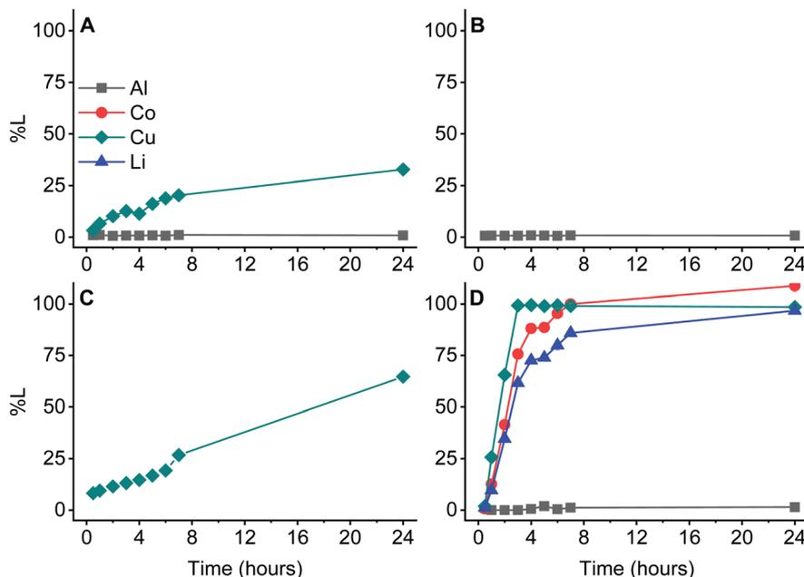
Fig. 7 Comparison of the leaching efficiencies by 75 vol% (diluted in an aliphatic diluent) D2EHPA during time of the current collectors solely. Only Al and Cu without LCO (A, left above), only Al without LCO (B, right above), only Cu without LCO (C, left below) and with Al and Cu with LCO (D, right below). Leaching parameters: 80 °C, 25 g L<sup>-1</sup>, 600 rpm. Al : LiCoO<sub>2</sub> = 12 wt%, Cu : LiCoO<sub>2</sub> = 24 wt%.
