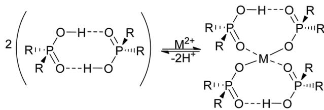
**Fig. 10** Simplified reaction of the coordination between D2EHPA (present as dimer) and divalent metal cations such as cobalt(II) and copper(II) during leaching.
