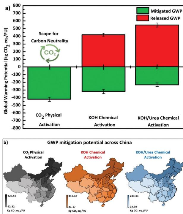
**Fig. 5** Global warming potential (GWP) impacts. (a) Comparison showing the released and mitigated GWP for the three activation methods; (b) potential GWP reduction across China under the CO<sub>2</sub> physical, KOH chemical, and KOH/urea chemical activation methods. Planning such WPDPC production units favors China, especially for the provinces whose GWP for electricity production is higher.
