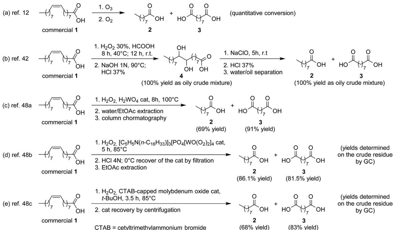
**Scheme 5** Known processes of oxidative cleavage of oleic acid (**1**) for the production of pelargonic (**2**) and azelaic acids (**3**) compared to that described in this work.
