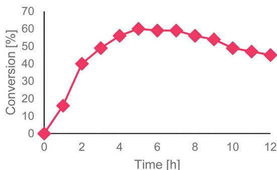
Fig. 2 Enzymatic conversion of oleic acid from hydrolyzed soapstock (by GC/MS) in the CSTR during 12 h of continuous operating time (samples progressively collected from the output of the reactor during the reaction course).
