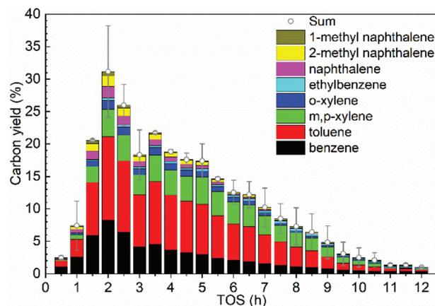
Fig. 1 Carbon yields of aromatics (BTX and others) *versus* TOS for a representative experiment (glycerol/oleic acid, 45/55 wt%, entry 11 in Table 1). Reaction conditions: H-ZSM-5/Al<sub>2</sub>O<sub>3</sub> (60/40 wt%) catalyst of 10 g, WHSV of the (co-)feeds of 1 h<sup>-1</sup>, N<sub>2</sub> flow of 50 ml min<sup>-1</sup>, reactor temperature of 550 °C, and atmospheric pressure.
