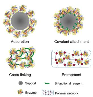
Fig. 3 The frequently used enzyme immobilization methods.
