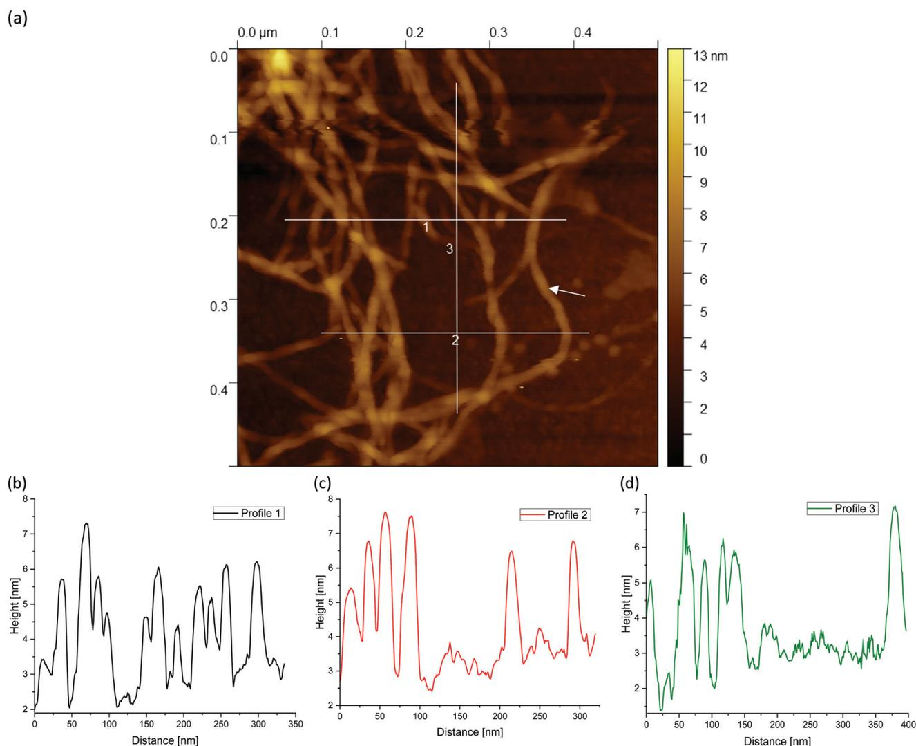
**Fig. 9** AFM image taken from the periphery of a (a) 0.5 wt% agarose fluid gel network with white lines showing the location of the corresponding height profiles (b–d) of the network structure. Number 2 is related to the horizontal line (image size = 0.5 × 0.5 μm).
