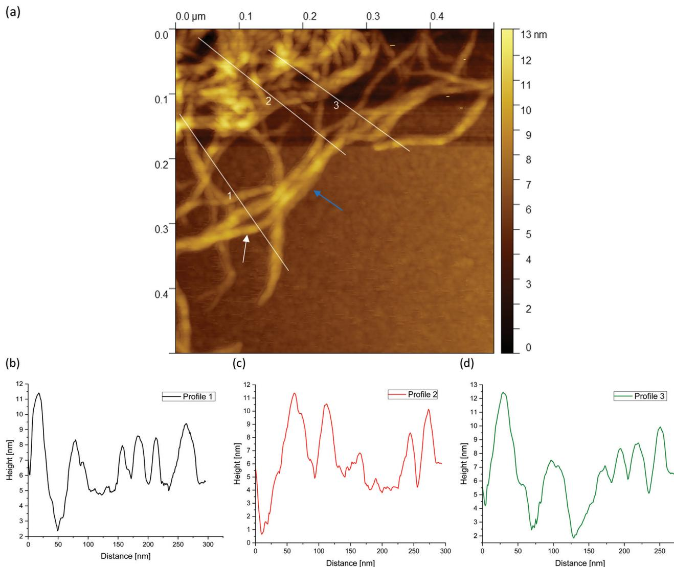
**Fig. 11** AFM image taken from the periphery of a (a) 2 wt% agarose fluid gel network with white lines showing the location of the corresponding height profiles (b–d) of the network structure (image size =  $0.5 \times 0.5 \mu\text{m}$ ).
