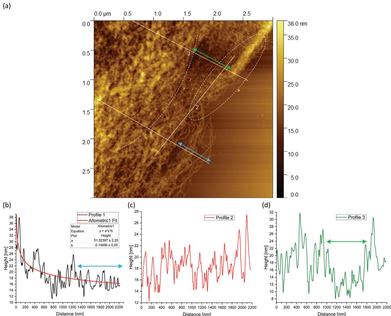
**Fig. 7** AFM image taken from the periphery of a (a) 2 wt% agarose fluid gel network with white lines showing the location of the corresponding height profiles (b–d) of the network structure. The green double arrow in (a) and (d) indicates thinning of the network structure, and the blue double arrow (a and b) indicates a partially ruptured network structure, both as a result of shear stresses during gelation (image size =  $3 \times 3 \mu\text{m}$ ).
