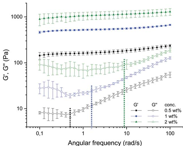
**Fig. 12** Frequency dependence of storage and loss moduli  $G'$  (filled symbols),  $G''$  (empty symbols) at a constant strain ( $\gamma = 0.05\%$ ) and temperature ( $T = 25\text{ }^\circ\text{C}$ ) for agarose fluid gels with different concentrations 0.5 wt% (black), 1 wt% (blue) and 2 wt% (green). The dashed lines indicate the angular frequency ( $\omega_c$ ) where  $G''$  starts to increase for the respective concentrations (reproduced from Ghebremedhin, Seiffert, and Vilgis<sup>7</sup>).
