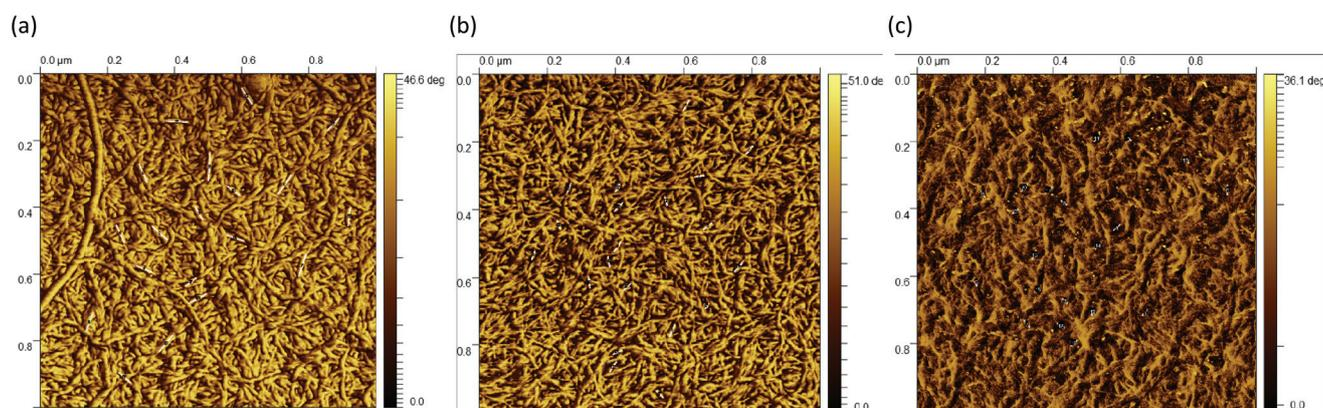
**Fig. 15** AFM phase images taken from the center (a) 0.5 wt%, (b) 1 wt% and (c) 2wt%. The indicated length was approximated to 48 nm for the 0.5 wt%, 27 nm for the 1 wt% and 18 nm for the 2 wt% fluid gel samples.
