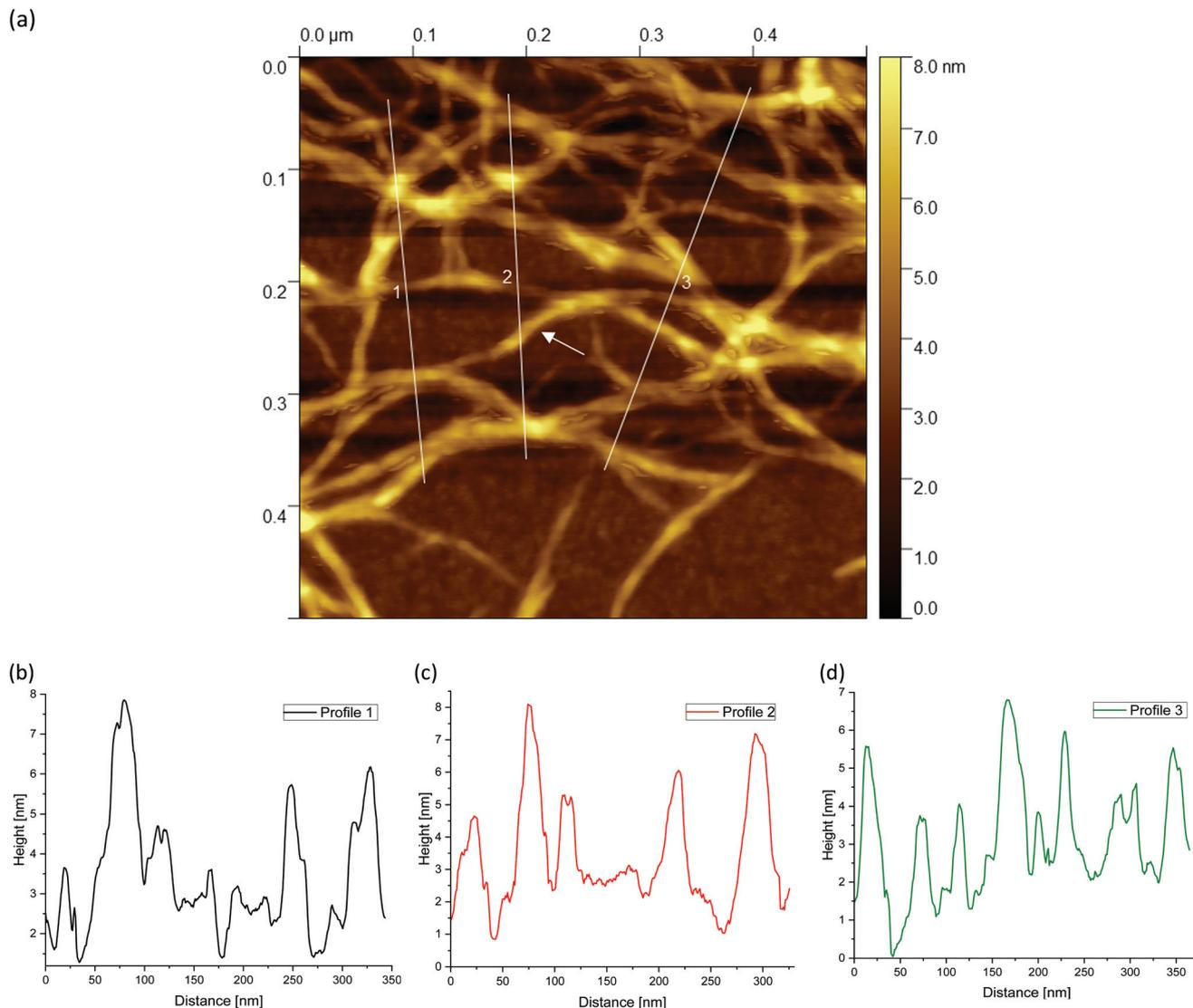
**Fig. 10** AFM image taken from the periphery of a (a) 1 wt% agarose fluid gel network with white lines showing the location of the corresponding height profiles (b–d) of the network structure (image size =  $0.5 \times 0.5 \mu\text{m}$ ).
