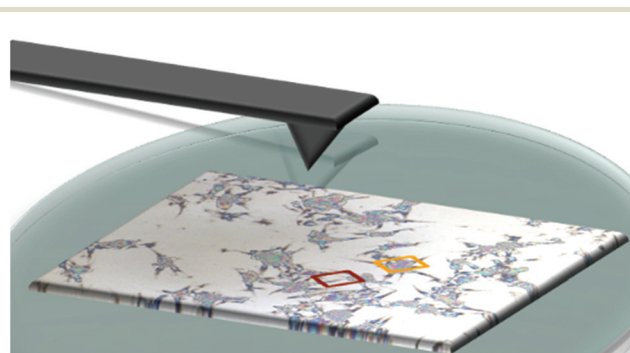
Fig. 1 A schematic illustration of the AFM experimental setup displaying the two different regions being investigated. Images were scanned from both the periphery (red), i.e. the chains on the particle surface, and the denser region (orange).
