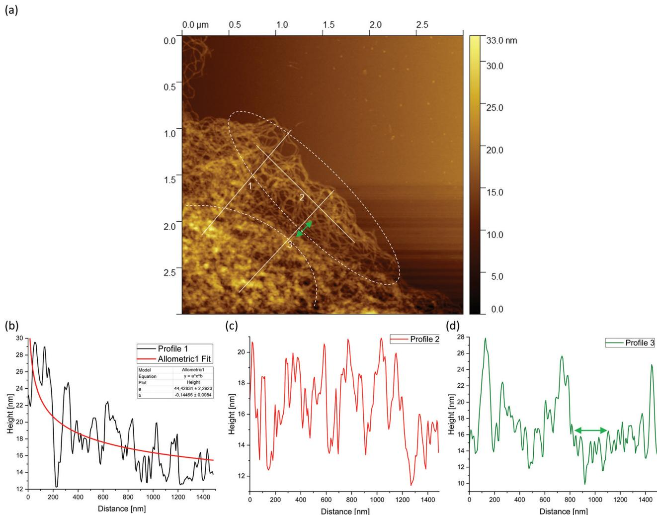
**Fig. 6** AFM image taken from the periphery of a (a) 1 wt% agarose fluid gel network with white lines showing the location of the corresponding height profiles (b–d) of the network structure. The green double arrow in (a) and (d) indicates the thinning of the network structure as a result of the microcracks formed during shear (image size =  $3 \times 3 \mu\text{m}$ ).
