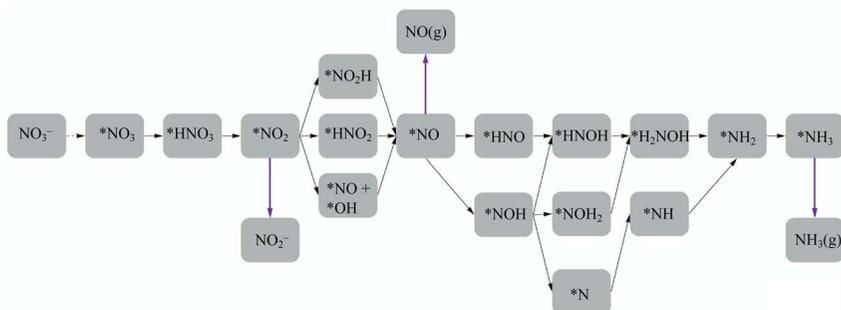
Fig. 2 Reaction paths and possible intermediates for the electrochemical reduction of  $\text{NO}_3^-$  to  $\text{NH}_3$  are considered in this work. Magenta arrows indicate the formation of nitric oxide ( $\text{NO}$ ), nitrite ( $\text{NO}_2^-$ ), and ammonia ( $\text{NH}_3(\text{g})$ ). The dashed arrow indicates a reaction with a proton transfer, and the solid arrows indicate reactions with a proton/electron pair transfer.
