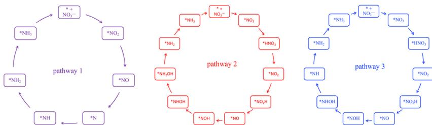
Fig. 3 Three different reaction pathways for the  $\text{NO}_3\text{RR}$  to ammonia on the Cu(111) surface reported by Hu *et al.*<sup>50</sup>
