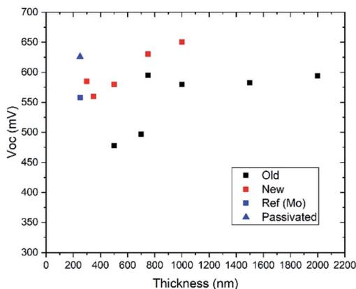
Fig. 1  $V_{OC}$  as a function of absorber thickness comparing published data (black) and new data (red), all on Mo back contact. Two devices (blue) from a different series using 250 nm thick CZTS comparing Mo and Mo/Al<sub>2</sub>O<sub>3</sub> back contact are also shown (see Table 2).
