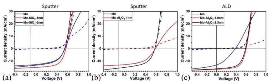
Fig. 3  $I$ - $V$  curves for devices with back contact passivation layers (a)  $\text{SiO}_2$  by sputtering, (b)  $\text{Al}_2\text{O}_3$  by sputtering and (c)  $\text{Al}_2\text{O}_3$  by ALD, compared to Mo reference devices.
