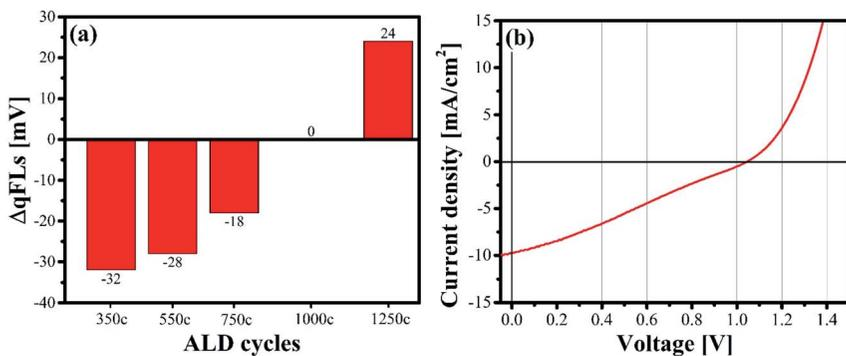
Fig. 4 (a) Bar chart showing the change in the qFLs of  $\text{Cu}(\text{In,Ga})\text{S}_2$  absorber before and after buffer deposition as a function of the  $(\text{Zn,Sn})\text{O}$  buffer thickness. (b) The characteristic  $J$ - $V$  curve of the  $\text{Cu}(\text{In,Ga})\text{S}_2$  device prepared with a 50 nm thick  $(\text{Zn,Sn})\text{O}$  buffer layer deposited at  $120^\circ\text{C}$ .
