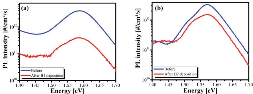
Fig. 1 (a) Absolute calibrated photoluminescence spectra of Cu(In,Ga)S<sub>2</sub> before and after (Zn,Sn)O buffer layer was deposited at (a) 105 °C (B1) and (b) 120 °C (B2), measured at an illumination intensity equivalent to one sun.
