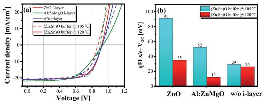
Fig. 2 (a) The characteristic *J*–*V* curves of the Cu(In,Ga)S<sub>2</sub> devices prepared with (Zn,Sn)O buffer layers deposited at 105 °C (B1) and 120 °C (B2), represented by dashed and solid lines respectively. The devices prepared with ZnO, Al:ZnMgO and without an *i*-layer are represented by red, green and blue lines, respectively. (b) Interface *V*<sub>OC</sub> deficit bar plot of devices made with B1 and B2 with various *i*-layer combinations.
