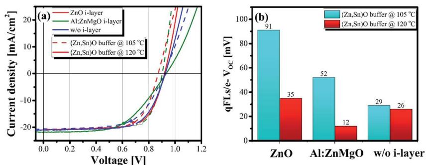
Fig. 2 (a) The characteristic *J*-*V* curves of the Cu(In,Ga)S<sub>2</sub> devices prepared with (Zn,Sn)O buffer layers deposited at 105 °C (B1) and 120 °C (B2), represented by dashed and solid lines respectively. The devices prepared with ZnO, Al:ZnMgO and without an i-layer are represented by red, green and blue lines, respectively. (b) Interface  $V_{\text{OC}}$  deficit bar plot of devices made with B1 and B2 with various i-layer combinations.
