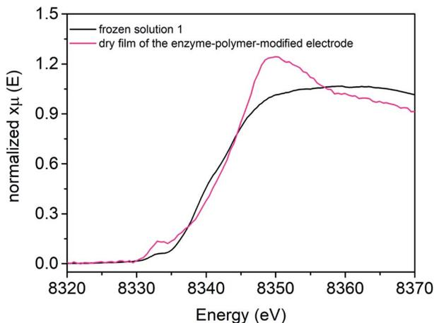
Fig. 4 Ni K-edge XAS spectra collected at 298 K at SAMBA Soleil beamline for a hydrogel film with [NiFe] hydrogenase from *DvMF* on GC electrode (pink line), and reference frozen solution of 1 (black line) measured at 10 K at SSRL 9-3 beamline.
