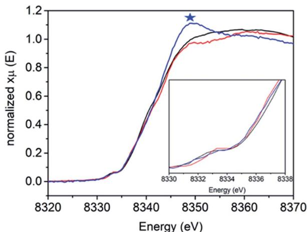
Fig. 3 Ni K-edge XAS spectra of [NiFe] hydrogenase from *DvMF* as isolated **1** (black line), incubated 4 hours with  $H_2$  **2** (red line) and reduced with NaDT/viologen **3** (blue line) measured at 10 K at SSRL 9-3 beamline. Blue asterisk corresponds to the energy edge at 8339 eV energy.
