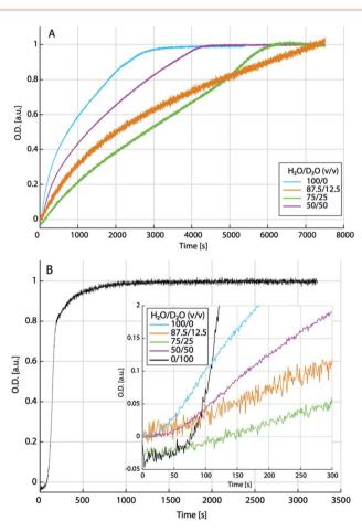
Fig. 6 Normalised transients extracted from the time development of the  $\nu_2$  carbonate vibrational band upon mixing 0.2 M calcium and carbonate solutions (liquid-liquid spinodal regime for pure light water) in different mixtures of light and heavy water as indicated (A); and in essentially pure (99.9%) heavy water (B). The inset in (B) shows a zoom into the early times of the transients shown in (A), together with the transient for heavy water.
