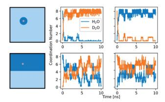
Fig. 7 Coordination number of  $H_2O$  and  $D_2O$  around a calcium ion. The rows show the results for two different setups. Top row: the ion with its first and second solvation shell is placed in the opposite solvent. Bottom row: the box is split into two compartments containing  $H_2O$  and  $D_2O$  and the ion is placed in one of them. Left: schemes of the initial setups. Middle: calcium ion initially surrounded by  $H_2O$ . Right: calcium ion initially surrounded by  $D_2O$ .
