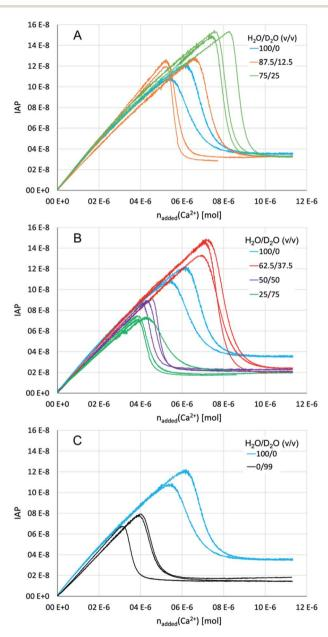
Fig. 5 Titration profiles for different  $H_2O$  and  $D_2O$  mixtures at an equivalent pH of 9.00 in pure water as indicated for (A) low heavy water contents; (B) high heavy water contents; (C) pure light vs. 99% heavy water. The data for pure light water is identical in panels (A), (B), and (C) so as to facilitate comparison. Individual repetitions are shown in the same respective colours, so as to illustrate reproducibility.
