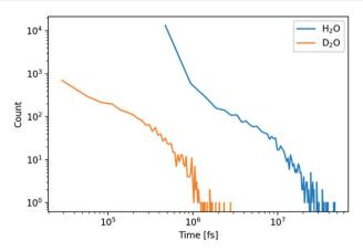
Fig. 3 Histogram of the lifetime of  $CaCO_3$  clusters containing more than 3 ions for simulations in  $H_2O$  and  $D_2O$  as indicated.
