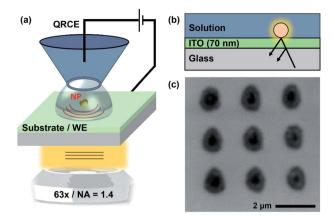
Fig. 1 Schematic (not to scale) of (a) the SECCM-IRM setup showing the SECCM probe, ITO WE and optical microscope. (b) Principle of operation of IRM to produce high contrast images of events and features at the WE interface. (c) Typical IRM image, recorded *in situ*, of an SECCM array section, with replicates of individual experiments. The darker electrolyte residue, left after probe retraction, is contrasted against the brighter ITO substrate background.
