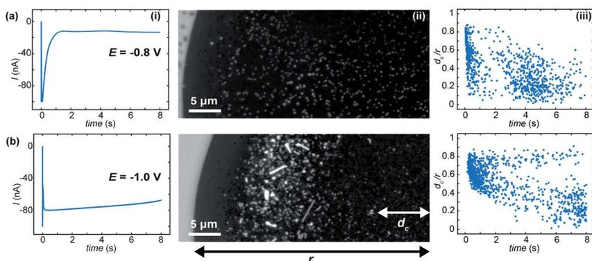
**Fig. 6** (i) SECCM current–time traces, (ii) IRM images and (iii) normalized radial position of new emerging optical features for the electrochemically-induced precipitation of  $\text{CaCO}_3$  at different applied potentials, within a *ca.*  $75\ \mu\text{m}$  wide meniscus. Applied potentials,  $E$ , (a)  $-0.8$  V and (b)  $-1.0$  V. IRM recordings captured a rectangular section of the meniscus (half of that shown here) at 200 FPS. Light source: blue LED (wavelength of  $470\text{ nm}$ ).
