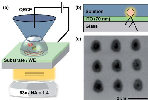
**Fig. 1** Schematic (not to scale) of (a) the SECCM-IRM setup showing the SECCM probe, ITO WE and optical microscope. (b) Principle of operation of IRM to produce high contrast images of events and features at the WE interface. (c) Typical IRM image, recorded *in situ*, of an SECCM array section, with replicates of individual experiments. The darker electrolyte residue, left after probe retraction, is contrasted against the brighter ITO substrate background.
