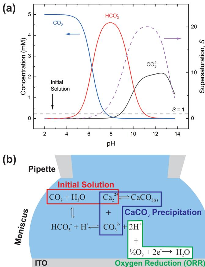
Fig. 4 The principle of electrochemically-induced  $\text{CaCO}_3$  precipitation. (a) Speciation diagram (left axis) and supersaturation (right axis) for the  $\text{CaCO}_3(\text{aq})$  system as a function of pH. Only principal species are shown, with the remaining mass balance made up of ion pairs (not shown). (b) Equilibria relating  $\text{O}_2$  reduction with  $\text{CaCO}_3$  precipitation.
