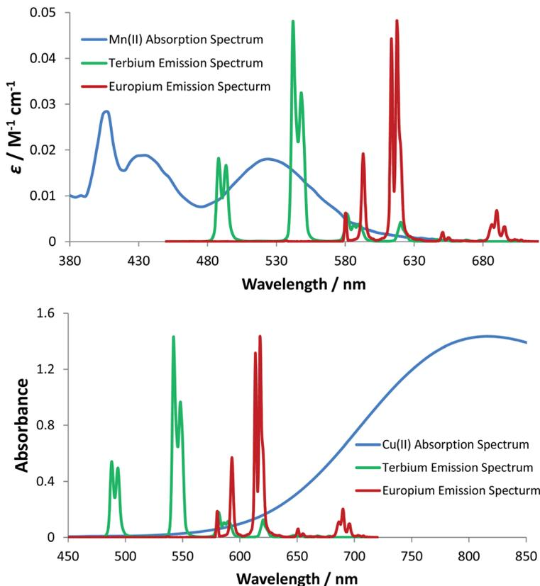
Fig. 6 (upper) Molar extinction coefficient for  $\text{MnCl}_2$  (blue) as a function of wavelength ( $\text{H}_2\text{O}$ , pH 7.4, 295 K); (lower) absorption spectrum of  $\text{CuCl}_2$  (blue) as a function of wavelength ( $\text{H}_2\text{O}$ , pH 7.4, 295 K). In each case, emission spectra for  $[\text{TbL}^{11}]$  (green) and  $[\text{EuL}^{11}]$  (red) are shown, permitting the analysis of the spectral overlap integrals.
