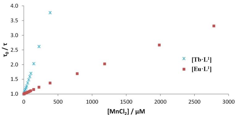
Fig. 5 Stern–Volmer plots for the quenching of  $[\text{EuL}^{10}]$  and  $[\text{TbL}^{10}]$  by  $\text{MnCl}_2$  ( $\text{H}_2\text{O}$ ,  $20 \mu\text{M}$  complex,  $0.1 \text{ M}$  HEPES,  $0.1 \text{ M}$  NaCl, pH 7.4,  $295 \text{ K}$ ).
