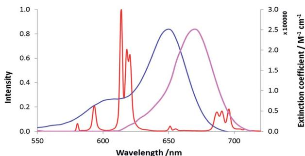
Fig. 4 Absorbance (blue) and emission (purple) spectra of the cyanine dye, **1**, compared to the [EuL<sup>7</sup>] emission spectrum (red), (MeOH, 295 K).
