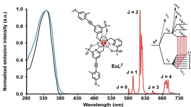
Fig. 2 Absorption (blue), excitation (black) and emission ( $\lambda_{\text{exc}}$  355 nm; red) spectra of [EuL<sup>2</sup>], showing the five major transitions to the  ${}^7F_n$  ground state from the europium  ${}^5D_0$  excited state, (295 K, 0.1 M NaCl).
