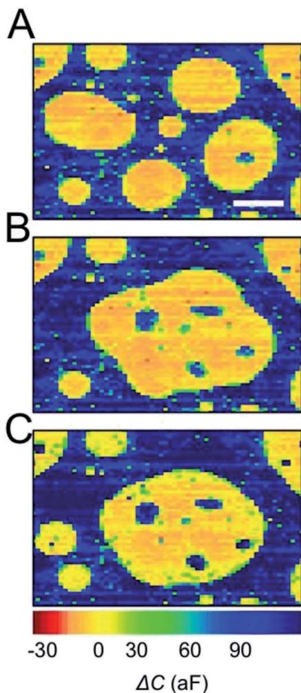
Fig. 5 Capacitance images of oDCB droplets taken at 0 s (A), 0.2 s (B) and 5.1 s (C). The scale bar is the same for all images and represents 10  $\mu\text{m}$ . The oDCB contains 1 mM of tetrabutylammonium toluene-4-sulfonate.
