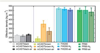
Fig. 6 The effective density ( $\rho_{\rm eff}$ ) of fresh and denuded 400 nm soot particles. The error bar indicates one standard deviation. Please note the y-axis origin.
