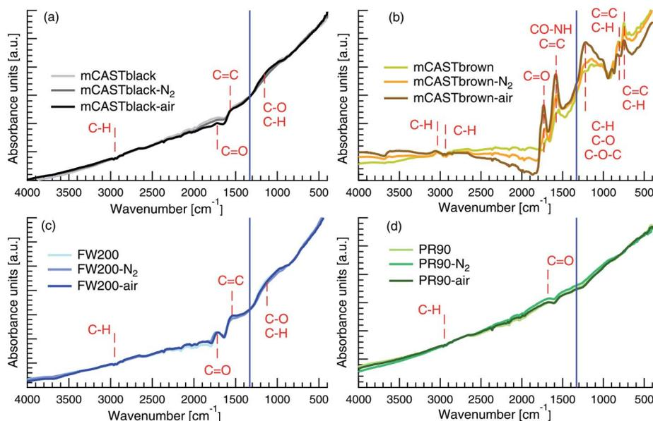
Fig. 5 Vector normalized ATR-AB (Attenuated Total Reflection-Absorption) spectra from FTIR measurements for fresh, oven-air ( $\text{N}_2 + \text{O}_2$ )- and  $\text{N}_2$ -heated soot. Likely chemical bond assignments are indicated in the individual spectra. The blue line corresponds to the wavenumber 1330  $\text{cm}^{-1}$  which separates the characteristic (left) and the fingerprint region (right).
