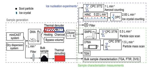
Fig. 1 Schematic of the experimental setup. miniCAST: miniature combustion aerosol standard; DMA: differential mobility analyser; CPC: condensation particle counter; HINC: horizontal ice nucleation chamber; OPC: optical particle counter; SMPS: scanning mobility particle sizer; CPMA: centrifugal particle mass analyser; TEM: transmission electron microscopy; TGA: thermogravimetric analyser; FTIR: Fourier transform infrared spectroscopy; DVS: dynamic vapour sorption.
