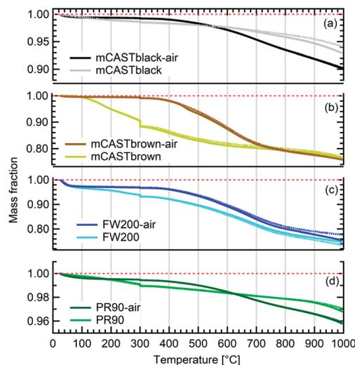
Fig. 4 TGA curves for fresh and oven-air-heated ( $\text{N}_2 + \text{O}_2$  atmosphere) bulk soot samples. Solid and dotted lines indicate two individual TGA runs. The  $T$  was held for 30 minutes at 300 °C. Red dashed line shows the bulk sample mass fraction benchmark, *i.e.*, 100%. Note the different y-axis scales for the samples.
