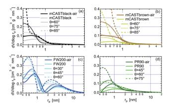
Fig. 8 The pore size distribution (PSD) as a function of pore radius  $(r_p)$ for fresh and synthetic air (N2 + O2) oven-heated soot with different contact angle assumptions, derived from DVS isotherms shown in Fig. 7. (a) mCASTblack, (b) mCASTbrown, (c) FW200, (d) PR90. In each panel, solid line, dotted line and dashed line indicate the PSD results of the same soot sample with different soot-water contact angle assumption values.
