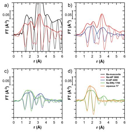
Fig. 6 Fourier-transformed  $k^2$ -weighted Tl L<sub>III</sub>-edge EXAFS spectra of Tl-containing Ba-muscovite, Tl-loaded Na-IdP and K-IdP, Na-SWy and of aqueous Tl<sup>+</sup>; sequentially pair-wise compared (a-d; thick lines indicate magnitude, thin lines imaginary part). Numbers in sample names indicate the Tl loading of the phyllosilicates in mg kg<sup>-1</sup>.
