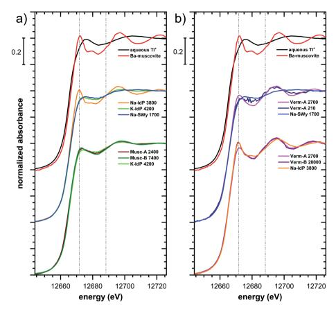
Fig. 5 Comparison of the Tl L<sub>III</sub>-edge XANES spectra of selected Tl-loaded phyllosilicate samples. Numbers in spectra labels indicate the Tl loading of the respective phyllosilicate in mg kg<sup>-1</sup>. Vertical lines serve to guide the eye. An enlarged version of figure focusing on post-edge oscillations is provided in Fig. S16.†
