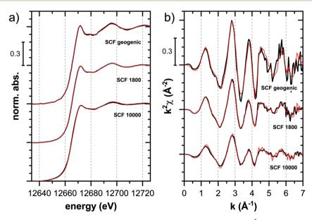
Fig. 8 Tl  $L_{\rm III}$ -edge (a) XANES and (b) EXAFS spectra of a soil clay fraction (SCF) with  $\sim$ 260 mg kg $^{-1}$  geogenic Tl (SCF geogenic) and with an additional 1800 mg kg $^{-1}$  (SCF 1800) or 10 000 mg kg $^{-1}$  freshly adsorbed Tl (SCF 10000) (black lines) and linear fit reconstructions (red lines). LCF results are listed in Table 2.
