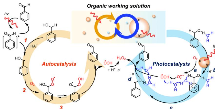
Fig. 6 Schematic of the mechanism of solar-driven H<sub>2</sub>O<sub>2</sub> production showing the interplay between auto- and photo-catalysis in an OWS.
